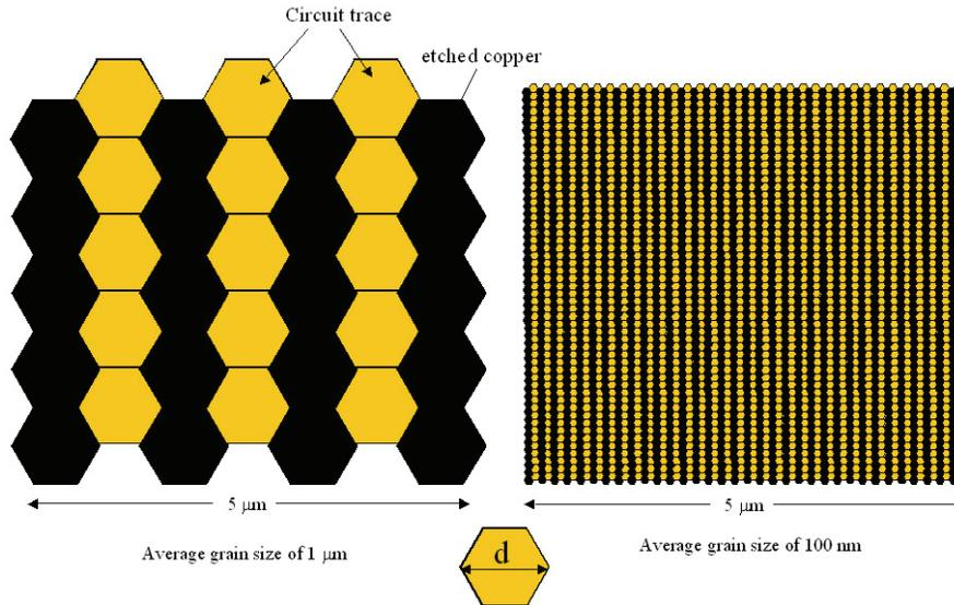
**Figure 1 – Schematic representation of PWB’s circuit trace after lithography and etching. Grain size reduction is expected to enhance trace resolution and achievable wiring density of the PWB.**
