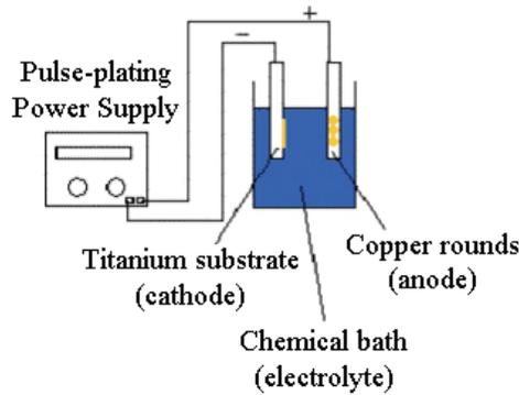
**Figure 2 – Schematic representation of pulse current electrodeposition setup**
