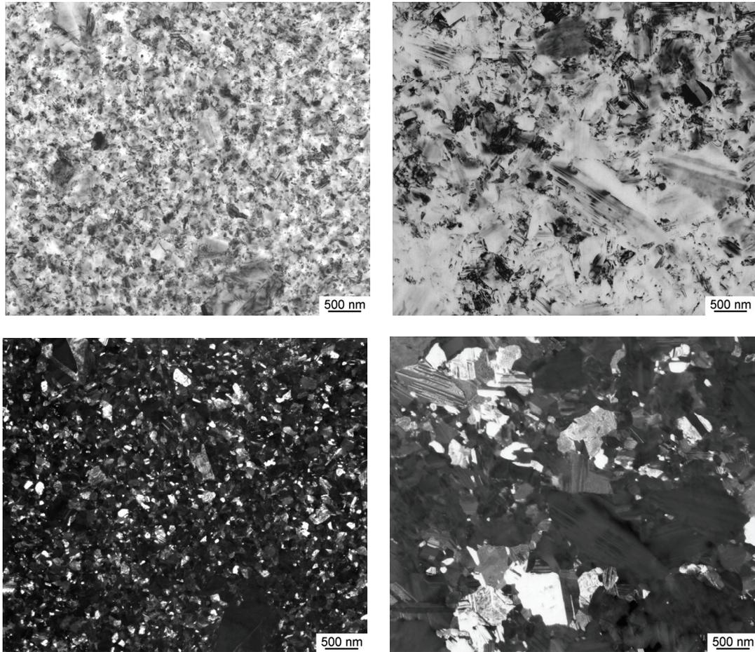
**Figure 3 – TEM bright field (top) and dark field (bottom) micrographs showing typical microstructures of electrodeposited nanocrystalline (left) and ultra-fine grain (right) copper.**
