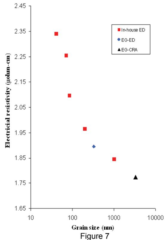
**Figure 6 and 7 – Dynamic hardness and electrical resistivity results for in-house and Commercially available copper foil as function of grain size.**
