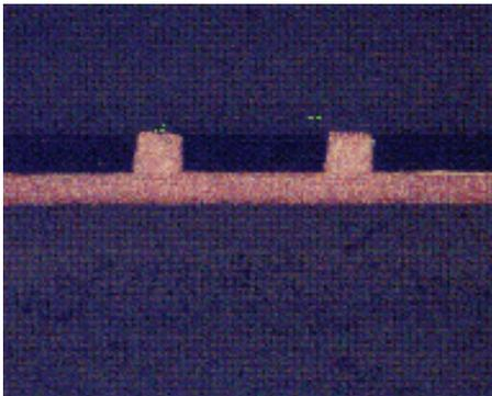
**Figure 13: 50.8  $\mu\text{m}$  Lines with 177.8  $\mu\text{m}$  Spaces.**
