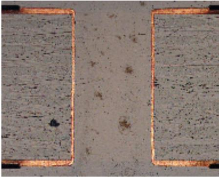
**Figure 11: 889  $\mu\text{m}$  Diameter PTH with Aspect Ratio of 1.7:1.**
