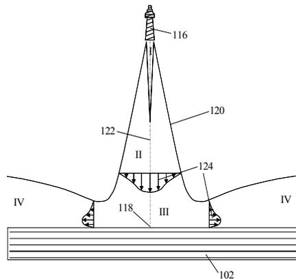
**Figure 3: Velocity Profile of Eductor Placed Perpendicular to PCB Surface.**<sup>17,18,19</sup>
