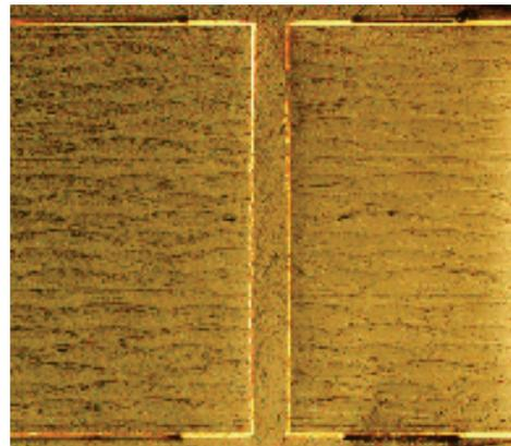
**Figure 18: 358.4  $\mu\text{m}$  Diameter PTH with Aspect Ratio of 10:1.**
