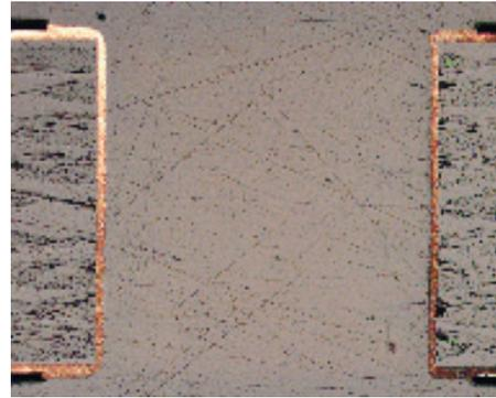
**Figure 12: 1600.2  $\mu\text{m}$  Diameter PTH with Aspect Ratio of 0.95:1.**
