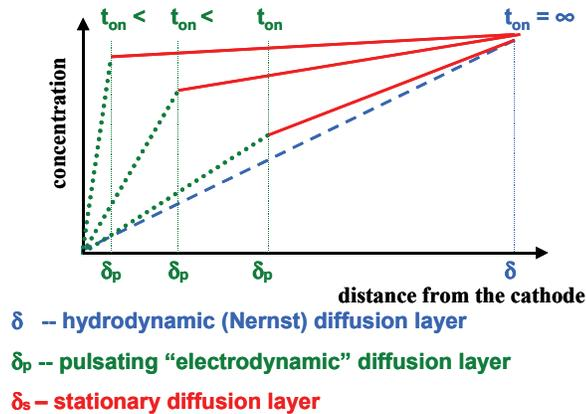
**Figure 2: Schematic Representation of the Duplex Diffusion Layer.**
