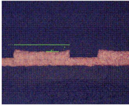
**Figure 16: 254  $\mu\text{m}$  Lines with 127  $\mu\text{m}$  Spaces.**
