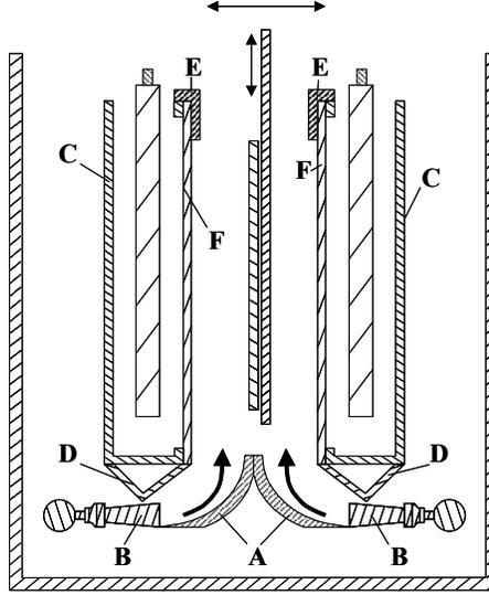
**Figure 4: Velocity Profile of Eductor Placed at an Angle to the PCB Surface.**<sup>20,21,22</sup>
