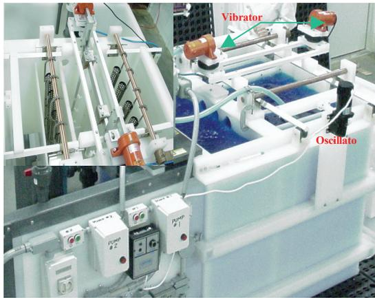
**Figure 6: Plating Cell.**
