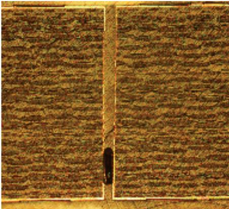
**Figure 17: 262.5  $\mu\text{m}$  Diameter PTH with Aspect Ratio of 15:1.**
