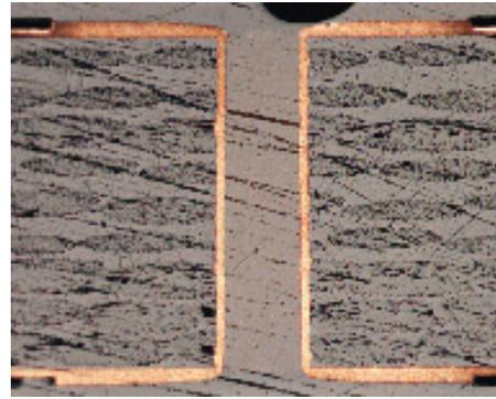
**Figure 10: A 609.6  $\mu\text{m}$  Diameter PTH with Aspect Ratio of 2.5:1.**
