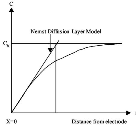
**Figure 1: Variation of the Concentration of the Reactant During Non-Steady-State Electrolysis.**
