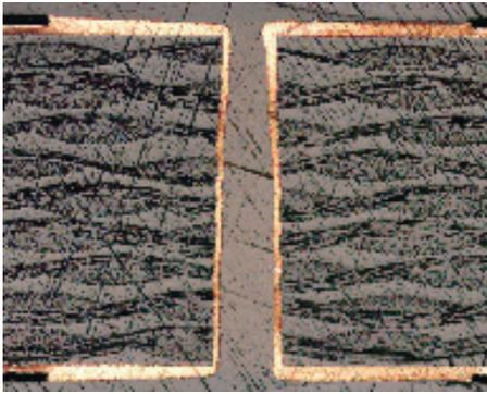
**Figure 9: A 330.2  $\mu\text{m}$  Diameter PTH with Aspect Ratio of 4.6:1.**
