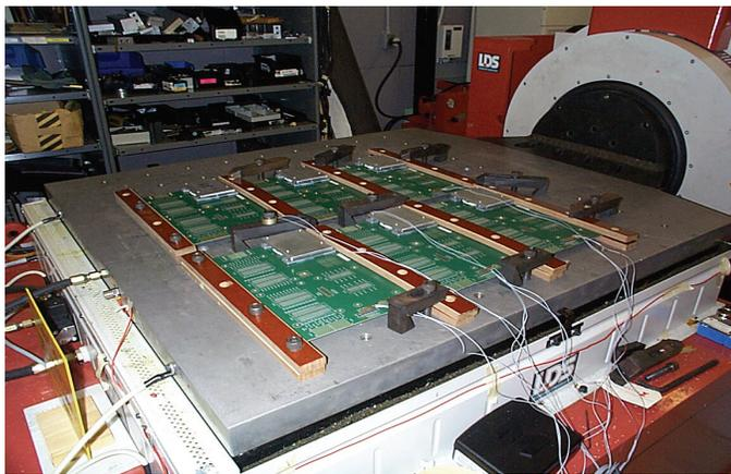
**Figure 10 - Setup of Vibration for X-axis**
