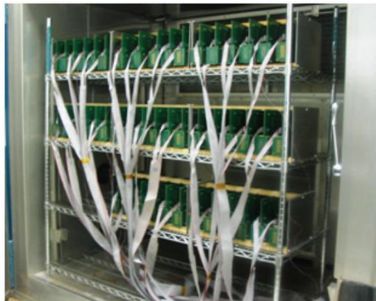
**Figure 7 - Assemblies in Thermal Cycling Chamber**
