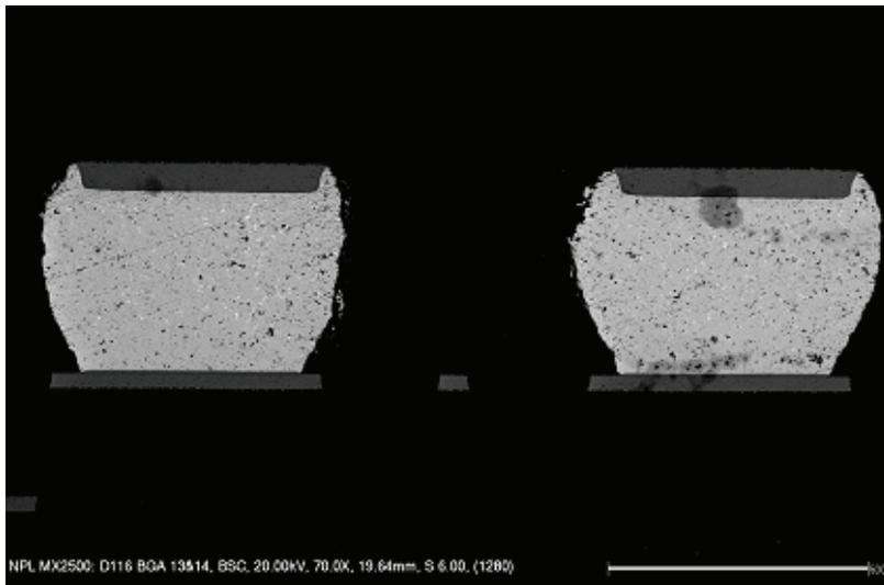
**Figure 12 - Section of Two Joints as Manufactured from SAC BGA Soldered with SnPbAg Solder Paste Showing Reflow of SAC Ball (PCB Uppermost) as Manufactured**
