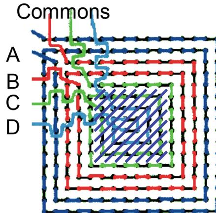
Figure 2 - Diagram of Daisy-Chaining within BGAs Showing Four Concentric Interconnected Rings (A, B, C and D), and a Hatched Area Representing The Location of The Component Eie
