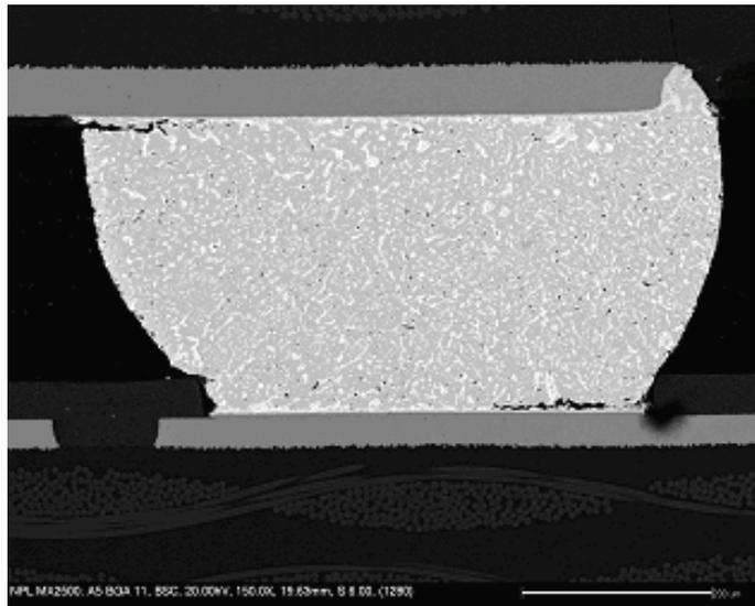
**Figure 13 - Section from Batch A (Tin-Lead BGA with SAC Solder) after 2000 Cycles Showing Fatigue Cracks at Both BGA/Solder and Solder/PCB Interfaces (PCB Uppermost)**
