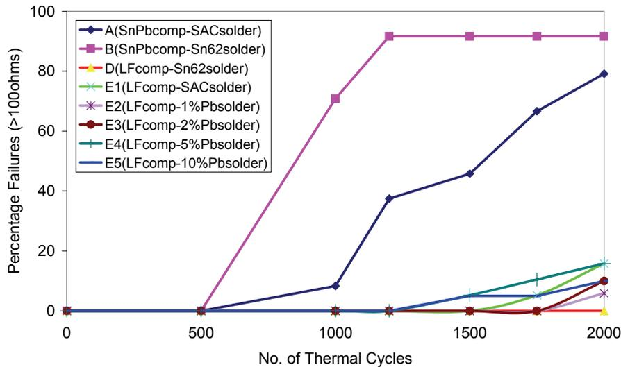
**Figure 11 - Development of BGA C-Ring Failures During Thermal Cycling**
