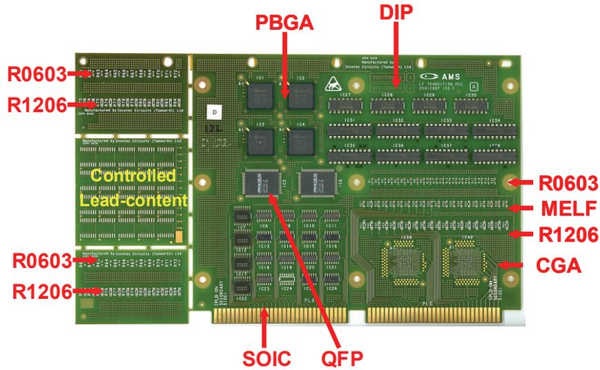
Figure 3 - TB64 Test Board
