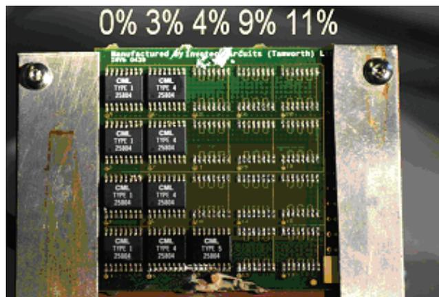
**Figure 14 - Lead-Contaminated Assembly after Inversion at 190°C Showing Loss of Lead-Contaminated Components after Sharp Tap (Annotated % Refers to Lead in Joint)**
