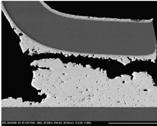
**Figure 10 - SEM Image of Micro-sectioned Sn-Plated QFP with SAC Alloy Joint after 2000 Thermal Cycles**
