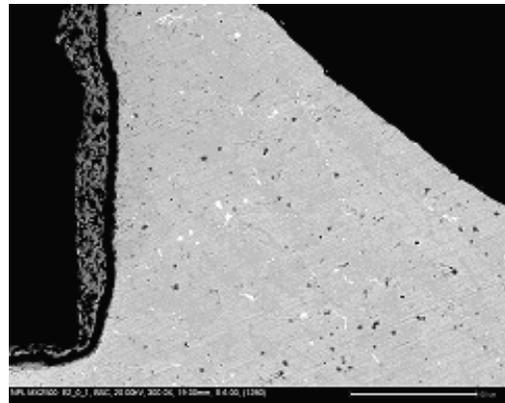
**Figure 5 - Micro-section of E2 Composition**
