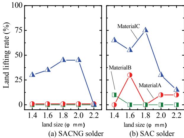
**Figure 4 - Correlation between Land Diameter and Land Lifting Rate After Soldering for Various Laminate Materials**
