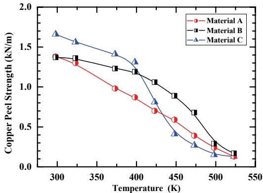
**Figure 9 - Temperature Dependence of Copper Foil Peel Strength**
