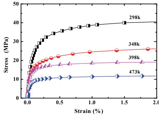
**Figure 7 - Stress-Strain Curves for SACNG Solder**
