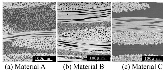
**Figure 2 - Cross Sections of The Three Laminates Differing in Inorganic Filler Content**
