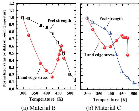
**Figure 10 - Temperature Dependence of Both Normalized Peel Strength and Land Edge Stress**
