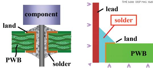
**Figure – 6 - Schematic Diagram of Stress Analysis Model**
