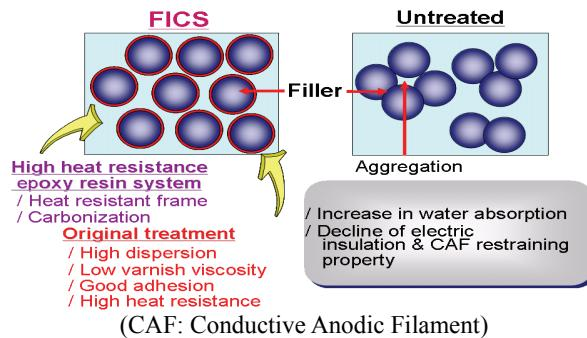
**Figure 1 - Schematic Diagram of Filler Interphase Control System**
