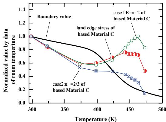
**Figure 11 - Temperature Dependence of Normalized Land Edge Stress for Modified Laminate Material C**
