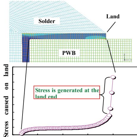
**Figure 8 - FEM Analysis of The Stress Caused on Land Field**
