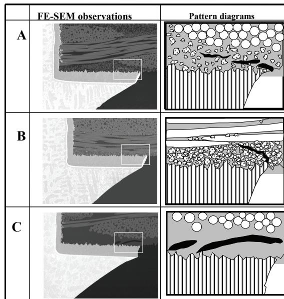
**Figure 3 - FE-SEM Images of Cross-Sections of The Fillet and The Cracking Pattern Diagrams of The Laminate Materials**
