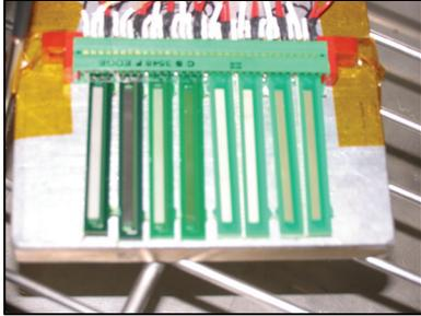
Figure 56a - SIR Mini Coupon Test Fixture
