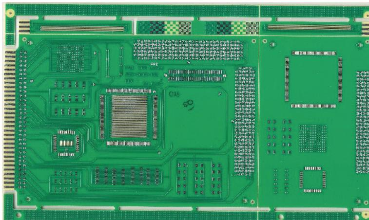
**Figure 5 - Prototype IPC-B-52 Test Boards**
