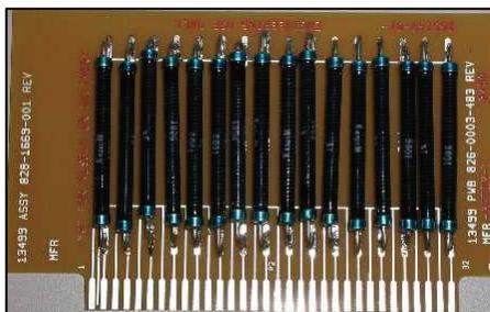
**Figure 35 - B52 Connector Checker Assembly**
