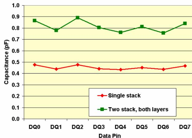
**Figure 7 - Comparing Capacitance Values for the Data Pins**
