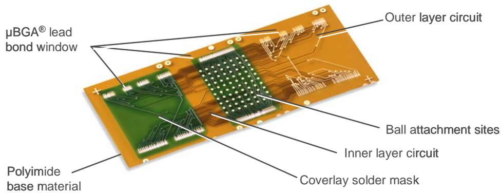
**Figure 2 - The Three Die Substrate Adapts 25 Micron Wide Circuit Conductors on Two Sides, Interconnected with Laser Ablated and Plated Micro-Vias**
