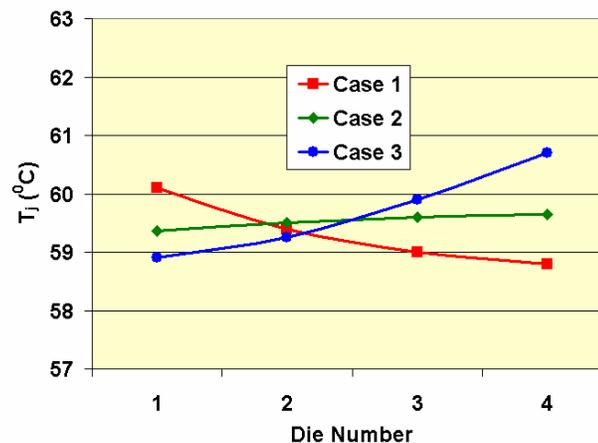
**Figure 8 - The Plot Illustrates the Variance of the Junction Temperature ( $T_j$ ) of the Die within the Four Die Ball Stack Package**
