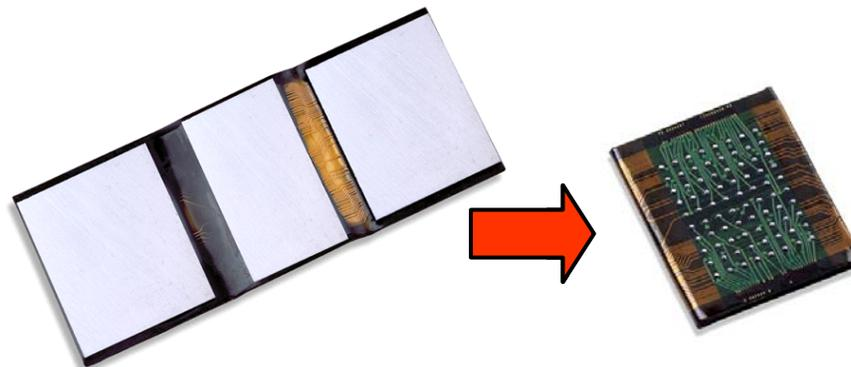
**Figure 1 - The Three Die µZ<sup>®</sup>-Folded Package Includes Two Flash Die and One SRAM Die, when Folded, Furnishes a Package Outline that is only Slightly Larger than the Largest Die in the Set**
