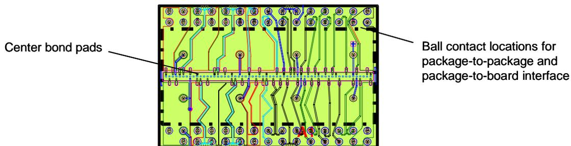
Figure 5 - The Substrate Designed for the Ball Stack Package for a Center-Bond Pad DDR Memory Die
