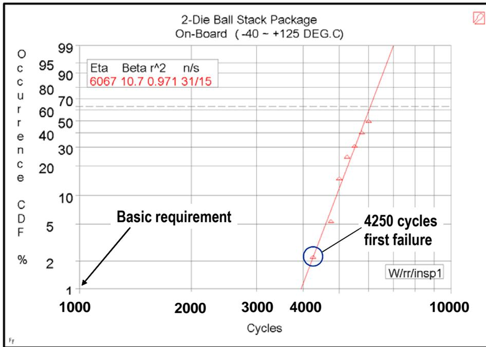
**Figure 10 - Weibull Plot for the Lead-Free Two Layer Ball Stack Package Recorded the First Failure in the Package Structure at 4250, Well Beyond the Basic 1000 Cycle Target**
