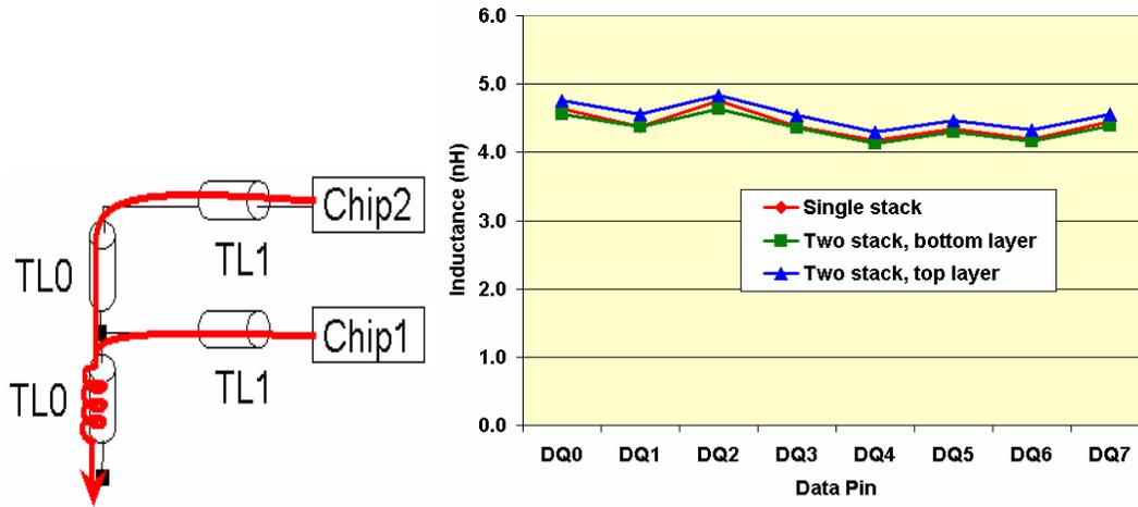
**Figure 6 - The Basic Inductance Circuit Model for Two Layer Ball Stack Package and the Graph Developed for Comparing Inductance Values for Eight Data Pins**
