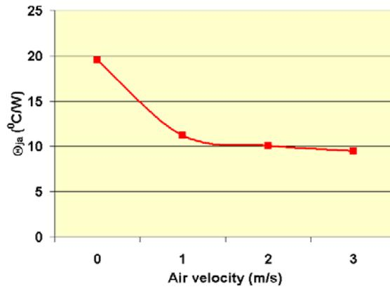
**Figure 9 - Package Thermal Resistance as a Function of the Air Velocity**
