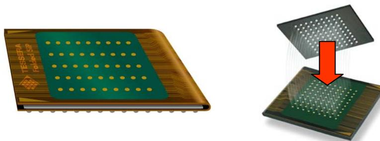
**Figure 3 - The Fold-Over Package Technology Provides a Land Pattern on its Top Surface to Accommodate the Stacking of Additional Packaged IC Devices**
