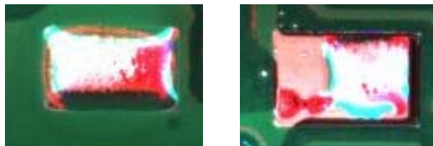
Figure 3 - Solder Pad Coverage. Photo to the Left Tin-Lead Solder, To the Right Lead-Free
