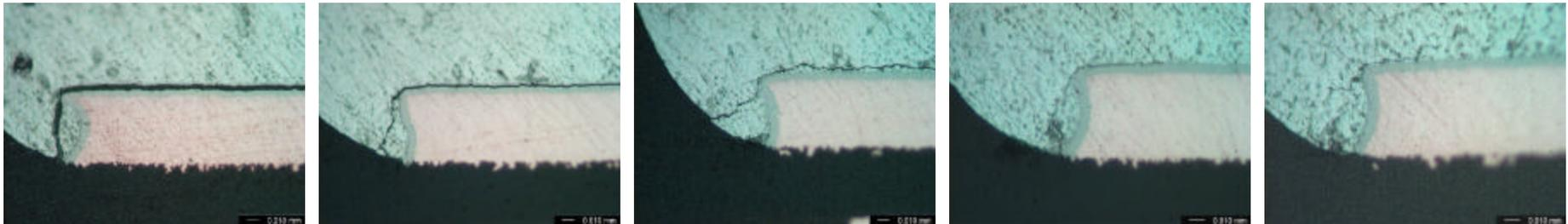
**Note: solder cracks at the left end of the PWB solder pad**
