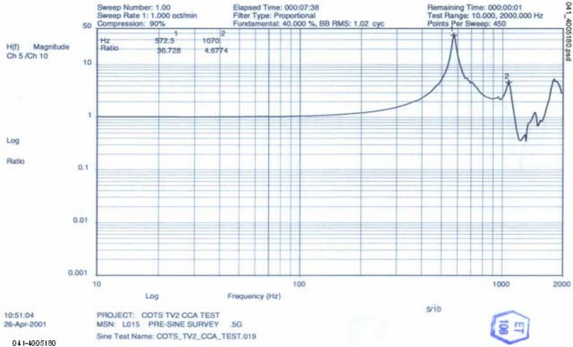
**Figure 4 – Typical Transmissibility Plot at the Center of the TV2 during a 1 g Sinusoidal Sweep**
