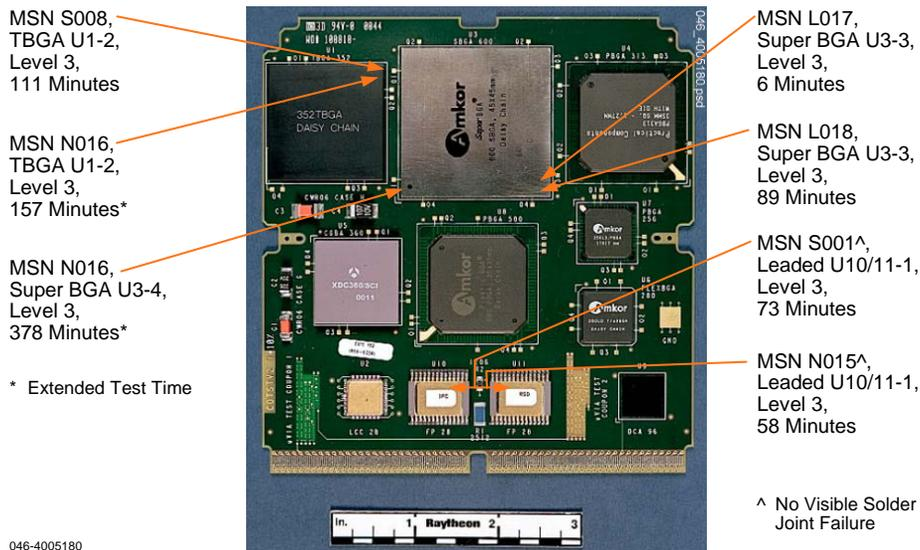
**Figure 5 – Failure Map of TV2 Random Vibration Test**
