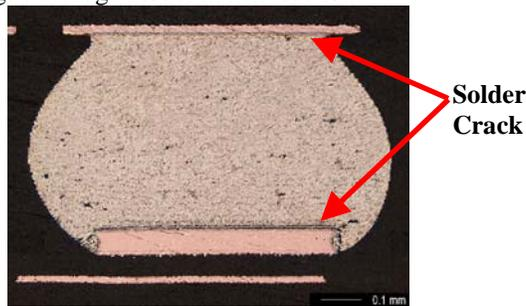
**Figure 6 – Microsection of Failed Solder Joint in 600-pin SBGA**
