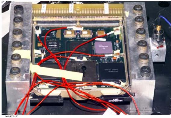
Figure 2 – TV2 Vibration Test Setup
