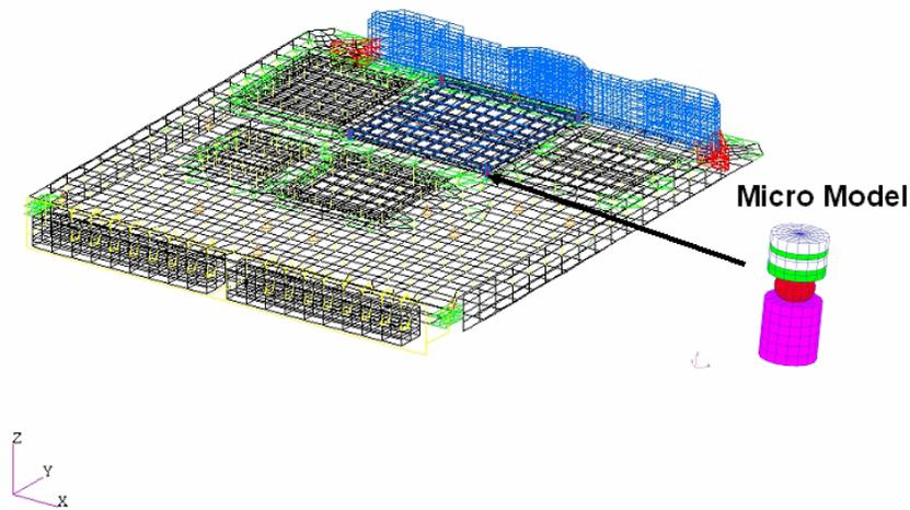
**Figure 7 – 3-D Macro/Micro Finite Element Model**
