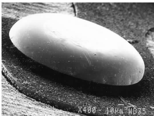
Figure 11 - Umbrella Shape Micro Bumps made by Plasma Etching
