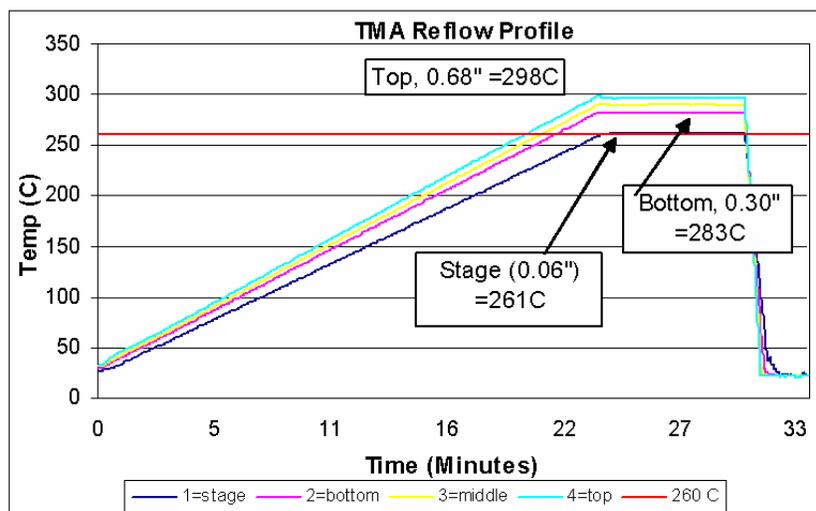
**Figure 5(a) - Temperature Readings from the Four Thermocouples Shown In Figure 4 during A T260 Test Run without Sample inside the Furnace Chamber**
