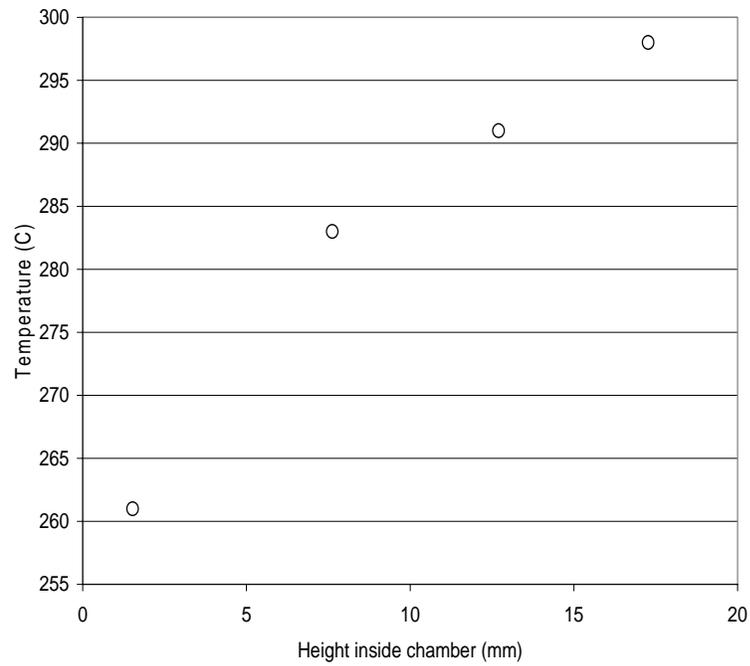
**Figure 5(b) - Peak Temperatures of the Four Thermocouples Shown In Figure 4, during a T260 Test Run without Sample inside the Furnace Chamber**
