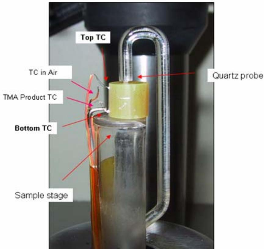
**Figure 2 - The Test Setup For Measuring The Temperature Gradient In A Laminate Sample. Two Tiny Thermocouples (tcs) are Embedded In the Laminate**
