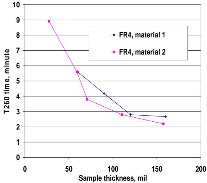
**Figure 1 - The Time to Delamination, Determined By TMA, Of a Printed Circuit Board Specimen at 260°C Decreases with the Specimen Thickness, Reported By Several Labs and With Several Fr4 Materials**
