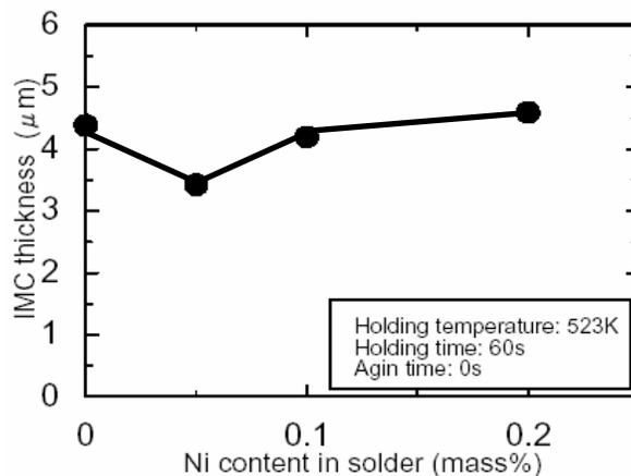
Figure 12 - Effect of Nickel in Tin-Copper Eutectic Solder on the Growth of Intermetallic on a Copper Substrate (Nishikawa et al<sup>2</sup>)
