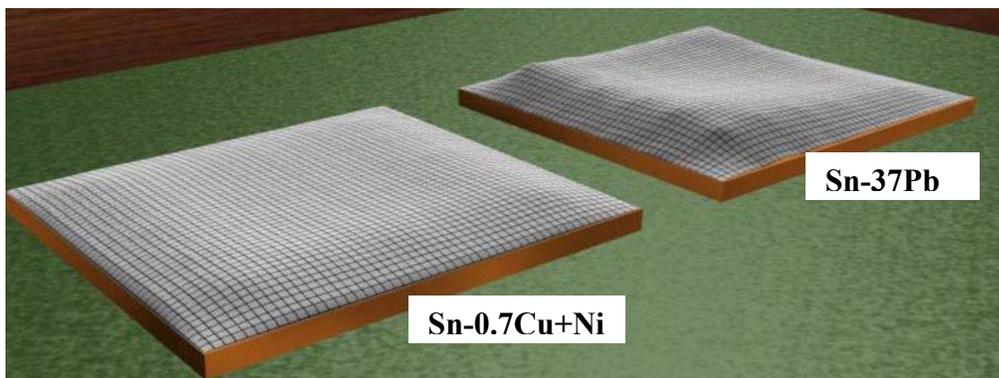
Figure 11- Improved Uniformity of HASL Coating Thickness of Nickel-Modified Tin-Copper Eutectic<sup>3</sup>
