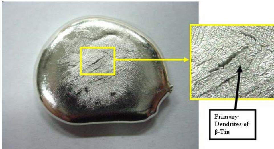
Figure 1- As Cast Structure of Unmodified Tin-Copper Eutectic
