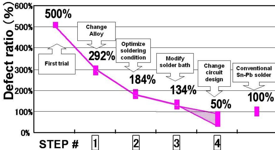
Figure 8 - Defect Rates during Implementation of Lead-Free Wave Soldering
