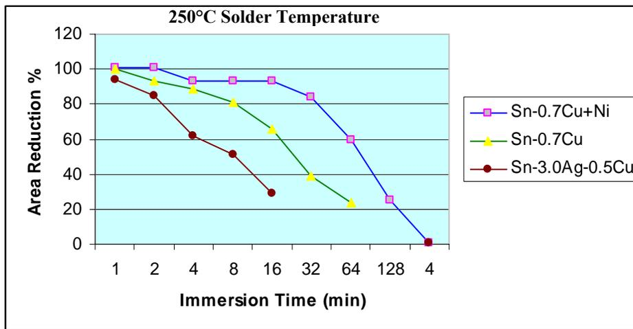
Figure 13 - Effect of Nickel Addition on the Copper Erosion Rate of the Tin-Copper Eutectic
