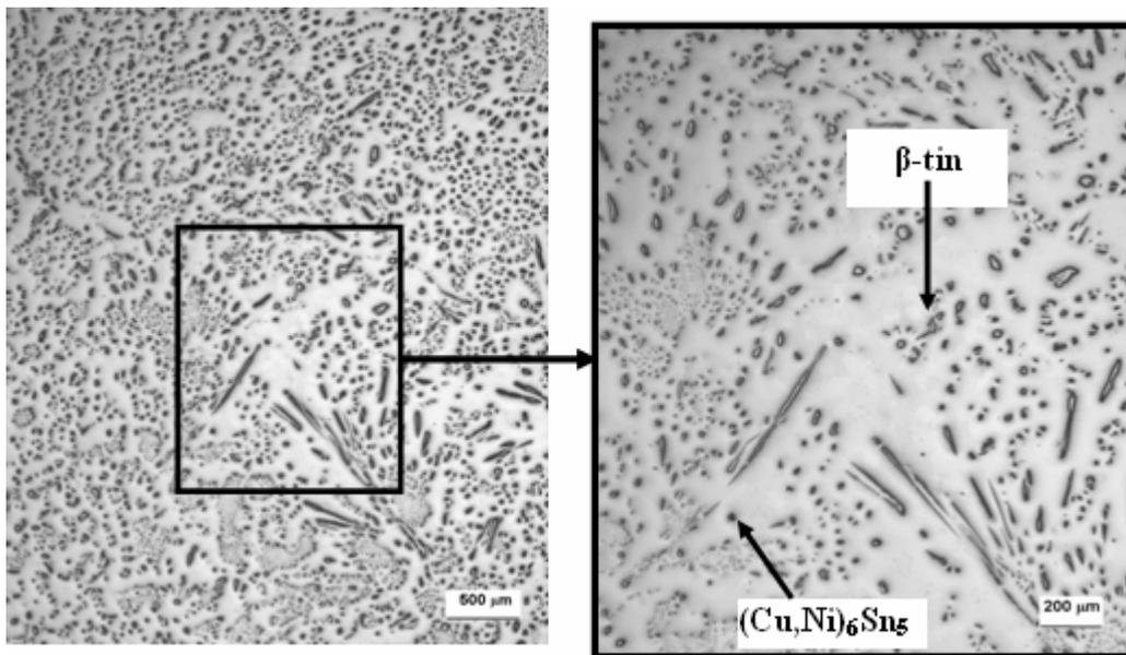
Figure 4 - Fully Eutectic Microstructure in Nickel-Modified Tin-Copper Eutectic
