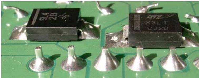
Figure 7- Smooth Bright Fillets Produced By Nickel-Modified Tin-Copper Eutectic
