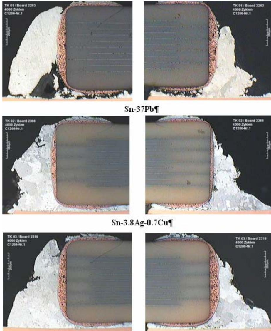
**Figure 14 - Performance of Nickel-Modified Tin-Copper Eutectic Solder Compared with Tin-Lead and Tin-Copper-Silver**
