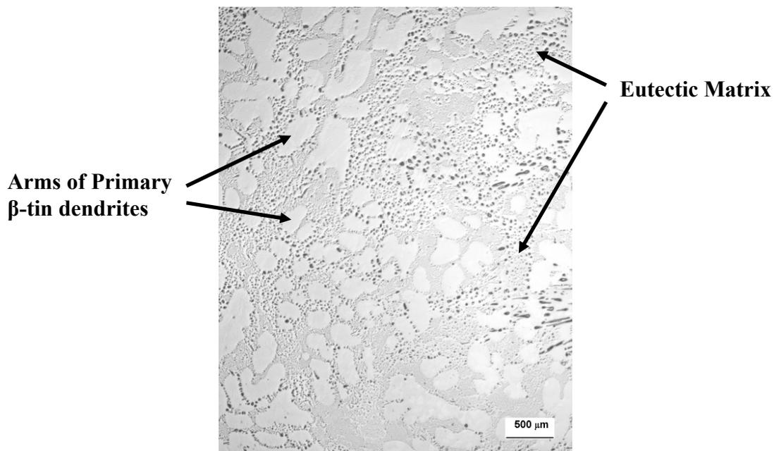
Figure 2- Microstructure of Unmodified Tin-Copper Eutectic
