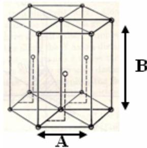
Figure 3 - Hexagonal Close Packed Crystal Structure of  $\text{Cu}_6\text{Sn}_5$  and  $\text{Ni}_3\text{Sn}_2$
