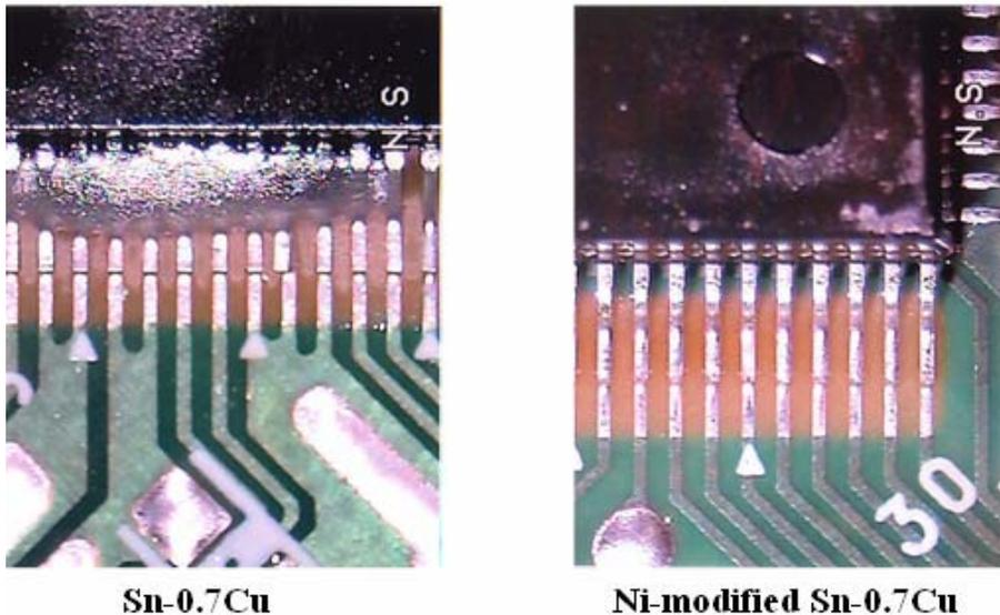
Figure 9 - Effect of Ni Addition on Bridging Behaviour of Sn-Cu Eutectic Solder
