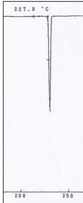
**Figure 6 - Differential Scanning Calorimetry Plot of Nickel-Modified Tin-Copper Eutectic**
