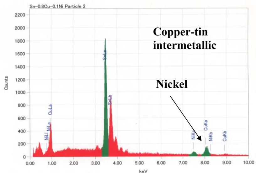
Figure 5 - Concentration of Nickel in the Copper-tin; Nickel Concentrates in the Intermetallic Phase
