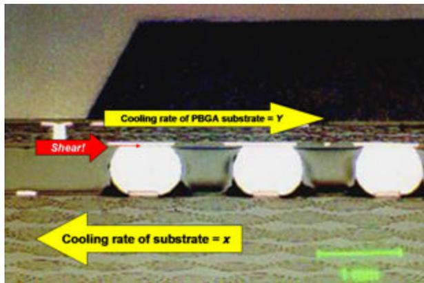
Figure 7 - Cross Section of BGA Revealing Shearing Zone
