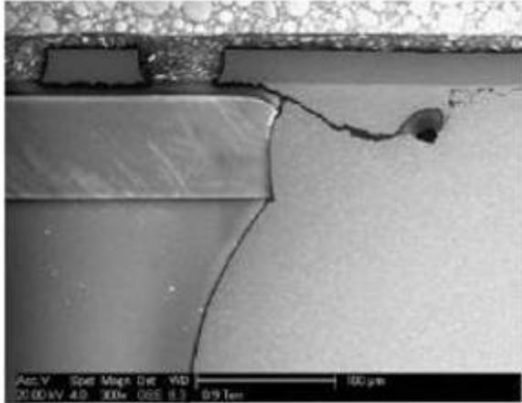
Failed Non-underfilled Assembly of Package H
