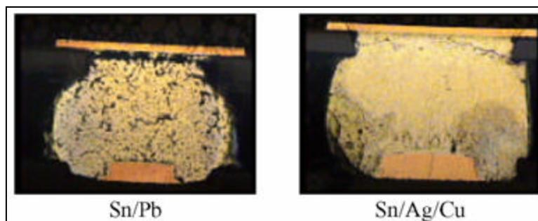
Figure 11 - Cracked Solder Joints for Sn/Pb and Sn/Ag/Cu Alloys due to Temperature Cycling
