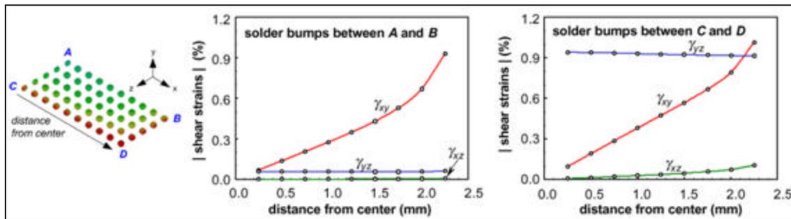
Figure 9 - Increased Shear Strain at Corner Balls
