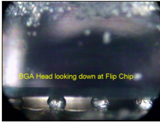
**Figure 13 - Standard BGA Optics Look Down at Bottom Fillet**
