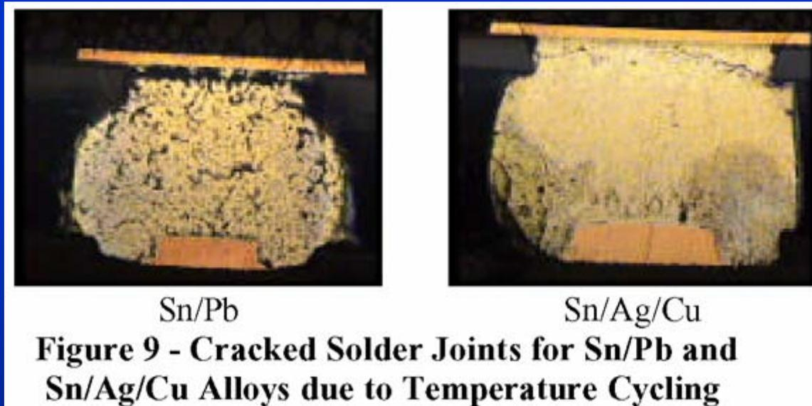
*“The failures reported above were analyzed with dye and pry and cross-sectioning techniques. Overall, it was found that solder joint failure for all of these Pb free alloys occur at the package side of the joint as is the case for Sn/Pb alloy. A representative x-section of joints with Sn/Pb and Sn/Ag/Cu alloys is shown in Figure 9.”*
