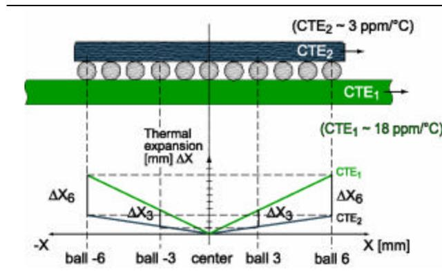
Figure 8 - Corner Balls are at Greater Risk Caused by CTE Mismatch during Cooling Delamination caused by CTE Mismatch
