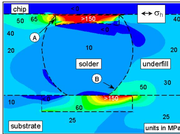
Figure 3 – Cell Analysis – Possible Failure Interface 1
