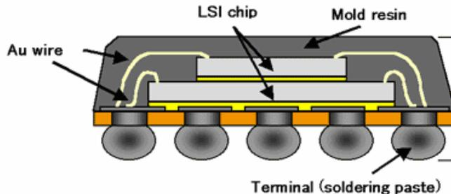
Figure 2 – Chip Scale Package
