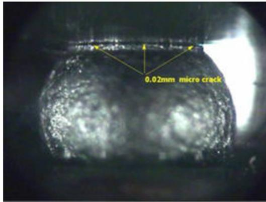
**Figure 22 – Top Side Delamination Visible**
