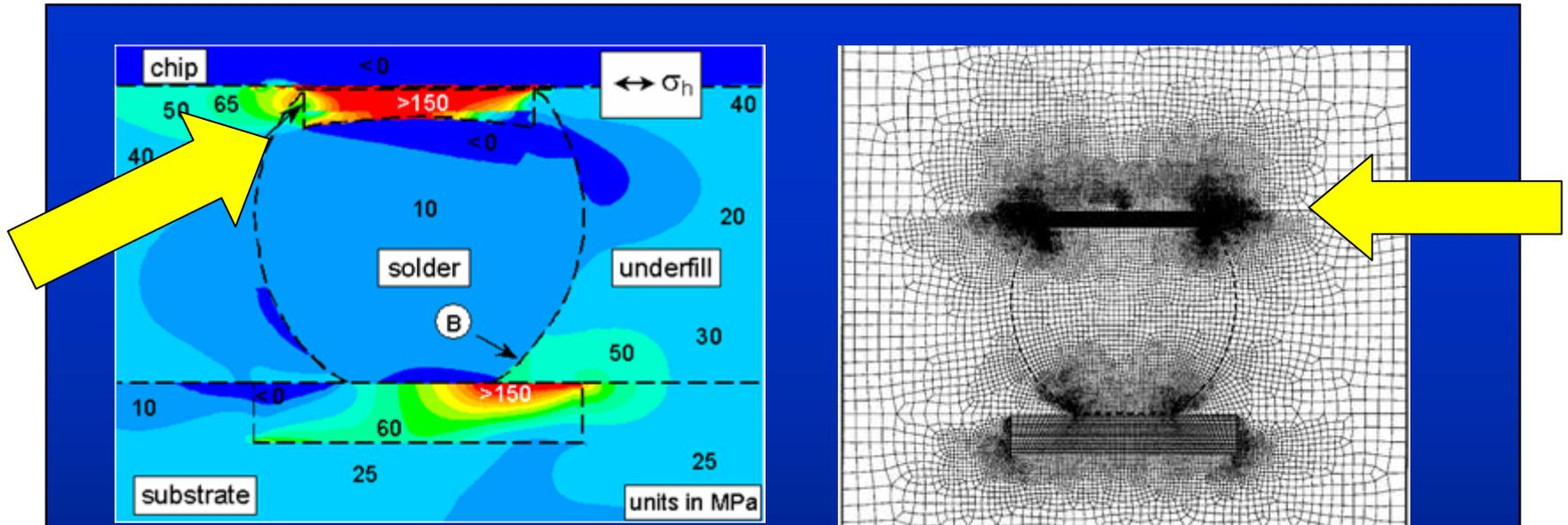
Professor Toshio Nakamura and Gary Yu Gu have conducted extensive research aimed at understanding the failure mechanism by identifying likely fracture modes and potential delamination sites in flip chip packages. Their research clearly shows that the upper solder connection is at greater risk of delamination as seen in the possible failure interface of the cell analysis figures above.
