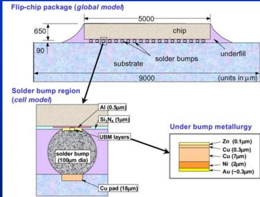
Source: 3D Interfacial Delamination Near Solder Bumps in Flip-Chip Package, by Yu Gu and Toshio Nakamura
