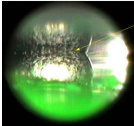
**Figure 17 – Corner Ball of BGA Delaminated**
