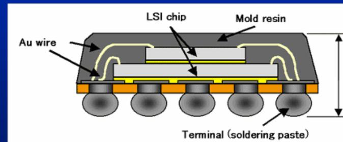
one fact remains; the size of the soldered connection is extremely small and is mechanically a weak point!
