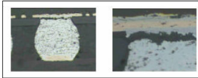
**Figure 12 - Typical failed SnAgCu Solder Joint Cross-Section**
