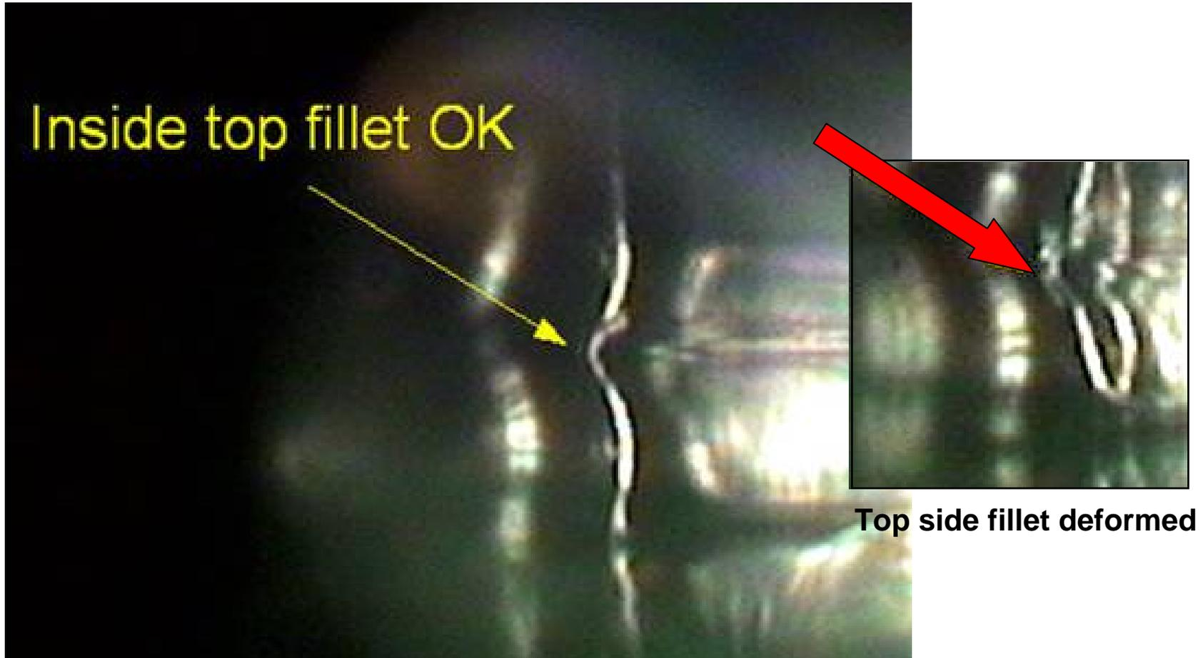
**Interior top side fillet inspection is possible with new Flip Chip optical head.**
