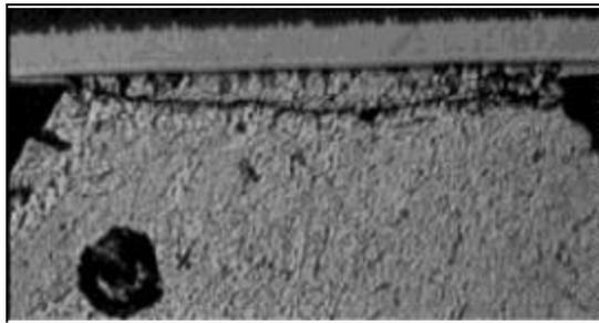
Figure 6 –Cross-sectional Image of Failed Package D Assembly (UF1)
