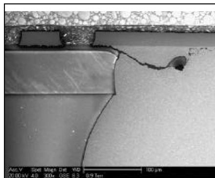
Figure 5 – Failed Non-underfilled Assembly of Package H
