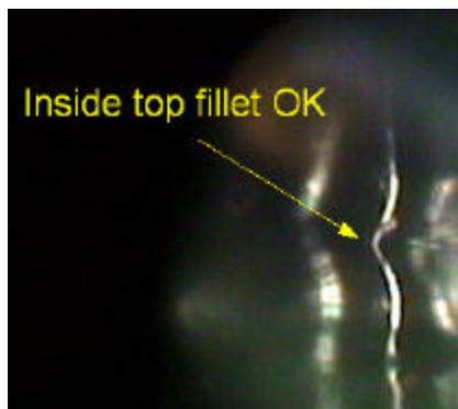
**Figure 18 – Interior top Side Fillet OK**
