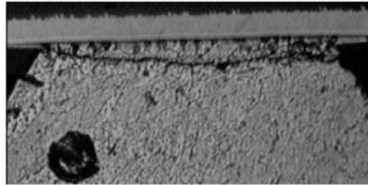
Cross-sectional Image of Failed Package D Assembly (UF1)
