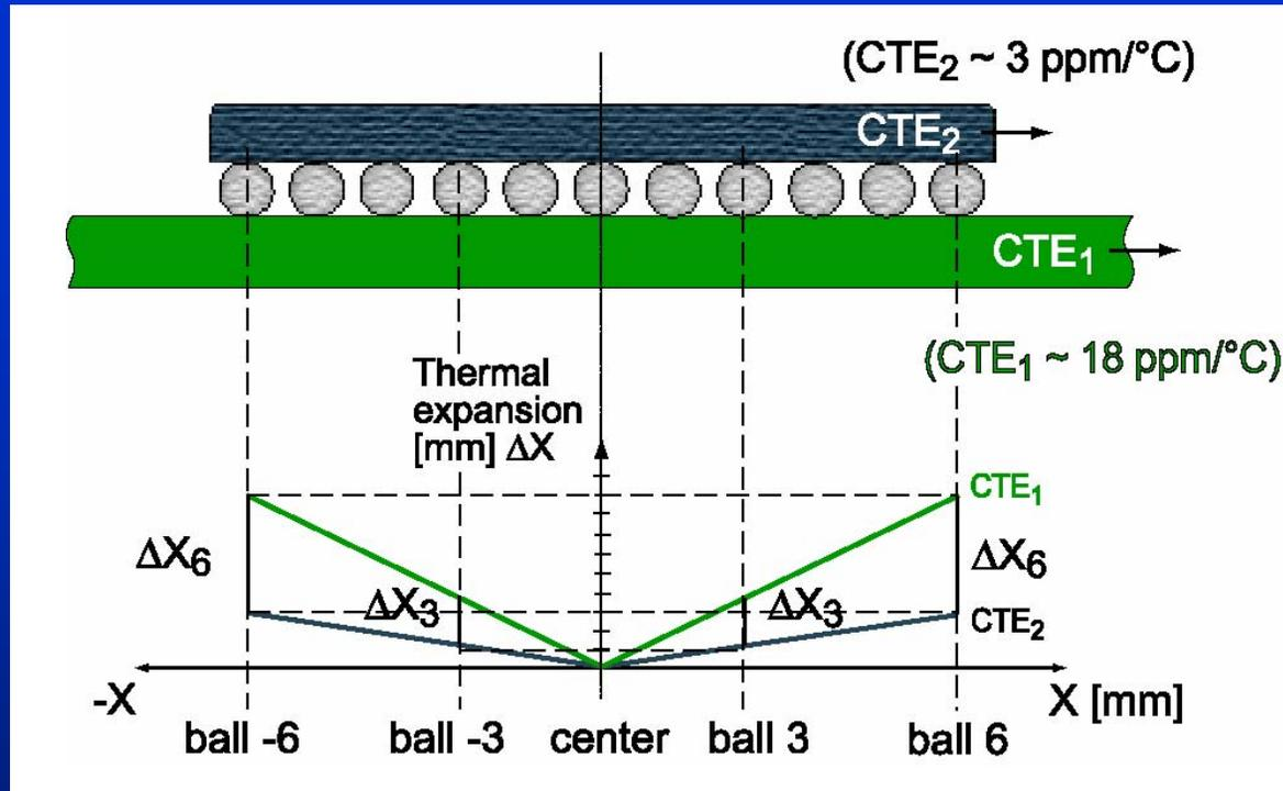
As we move towards the corners of the package, the relative movement differential increases as the distance from the center point increases. This stress is substantially larger at the corners of the component and can result in increased micro crack formation at the corner joints.
