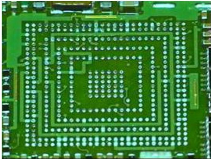
**Figure 7 - BGA Pads 0.3 mm after Package Removal**
