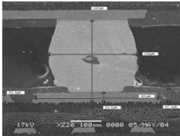
**Figure 6 – BGA Solder Joint – Mask Defined Pads**
