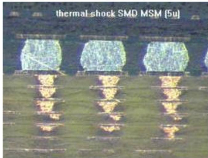
**Figure 11 - X-sections Post Thermal Shock**
