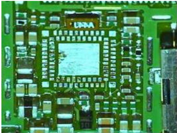
**Figure 8 - BCC Pads after Package Removal**
