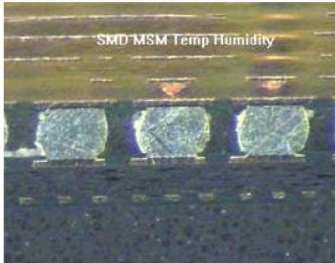
**Figure 10 – X-section Post Temp. Humidity**
