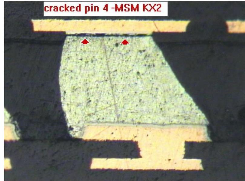
**MSM Pin Cracks - No
