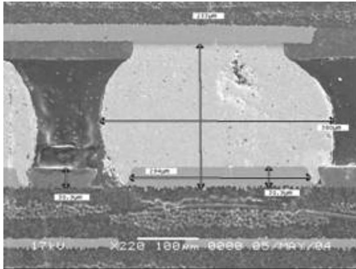
**Figure 5 - BGA Solder Joint- Etch Defined Pads**
