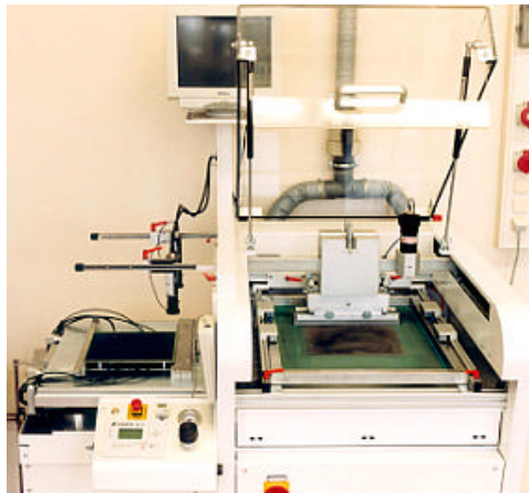
Figure 16 - Batch Type Screen Printer used in Fuel Cell Manufacturing Today
