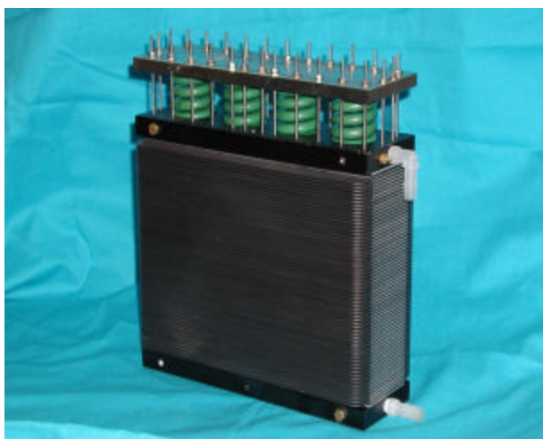
Figure 6 - Fuel Cell Stack (PEM, 700W, 65 Cells)
