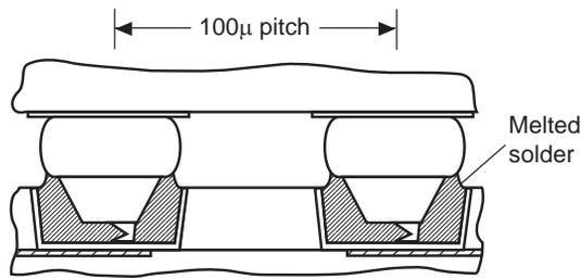
**Figure 13(b) - Completed Bump/Well Connection**
