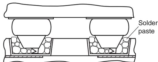
**Figure 13(a) - Stud Bumps are Inserted into the Wells**
