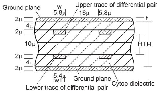
**Figure 14,  $Z_{diff} = 100\Omega$  - Broadside-Coupled Stripline**
