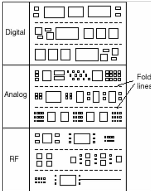
**Figure 19 - Circuit Assembly wherein the Signal Types are Separated for Convenience and Electrical Isolation**
