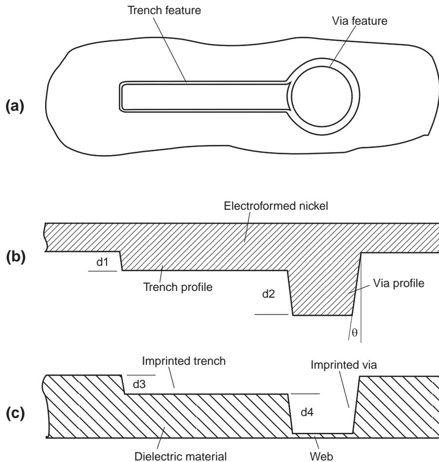
**Figure 6 - Basic Imprinting Geometries**
