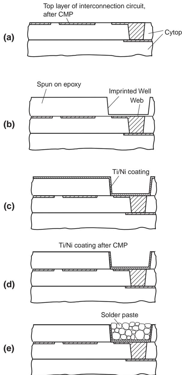
Figure 8 - Imprinting and CMP Provide an Effective and Inexpensive Way to Create the Wells
