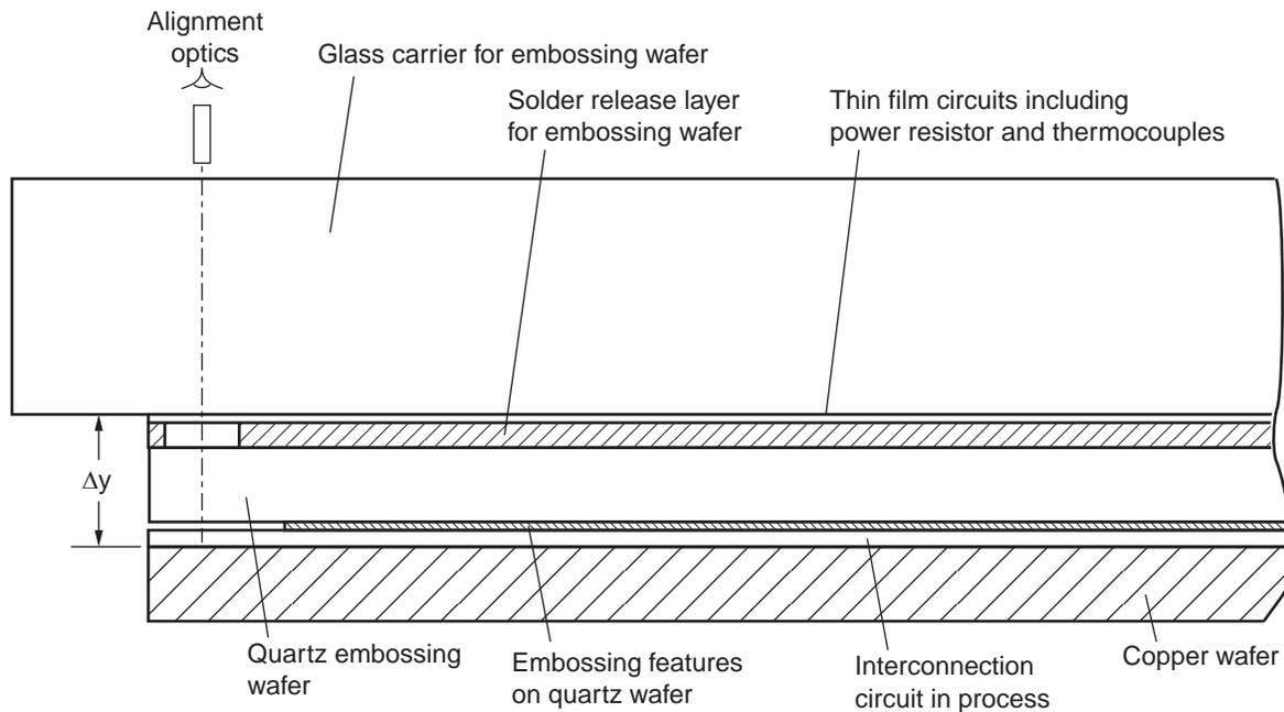
**Figure 1 - A Schematic of an Alignment Stack**
