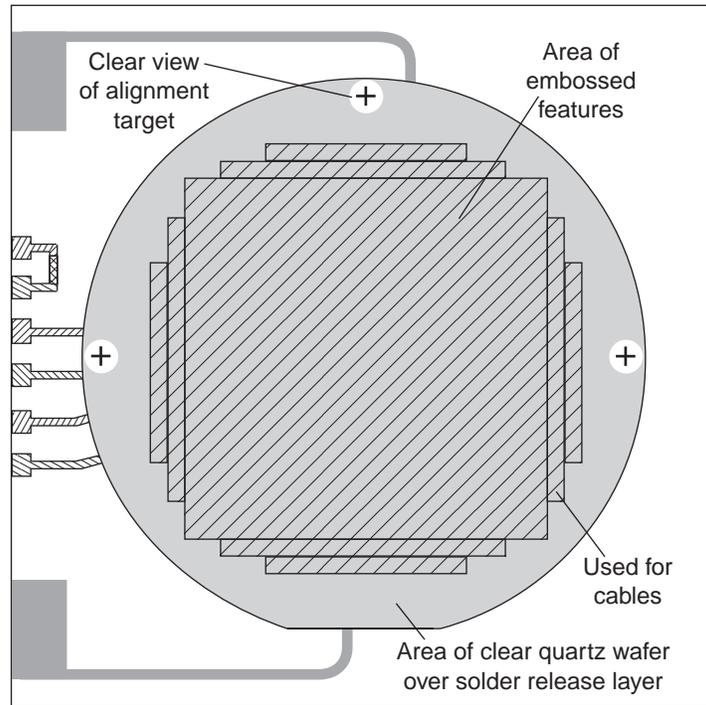
**Figure 5 - Embossing Tool, after Bonding the Quartz Wafer to the Glass Carrier**
