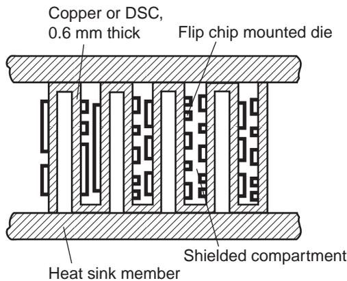
**Figure 20 - One Possible Arrangement for Folding the Circuit Assembly and Providing Good Heat-Sinking Capability**
