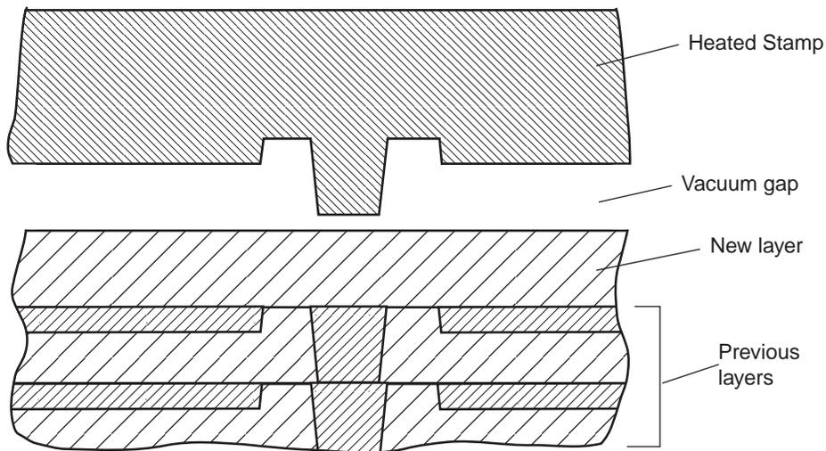
**Figure 10 – Heating of the Top Layer of the Dielectric Stack**
