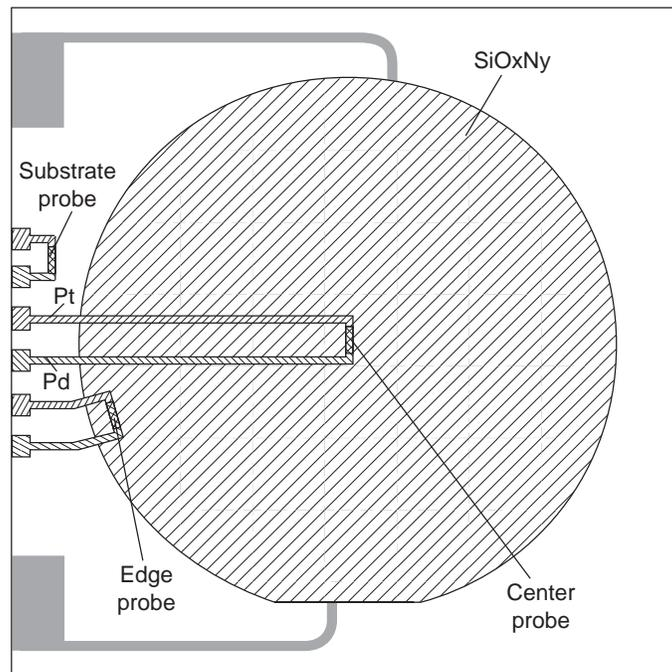
**Figure 4 - Coating of Silicon Oxy-Nitride**
