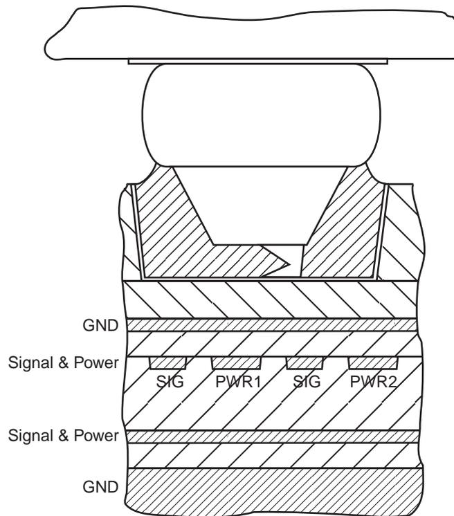
**Figure 17 – Reduction in Imprinted Layers with Power Mesh Architecture**
