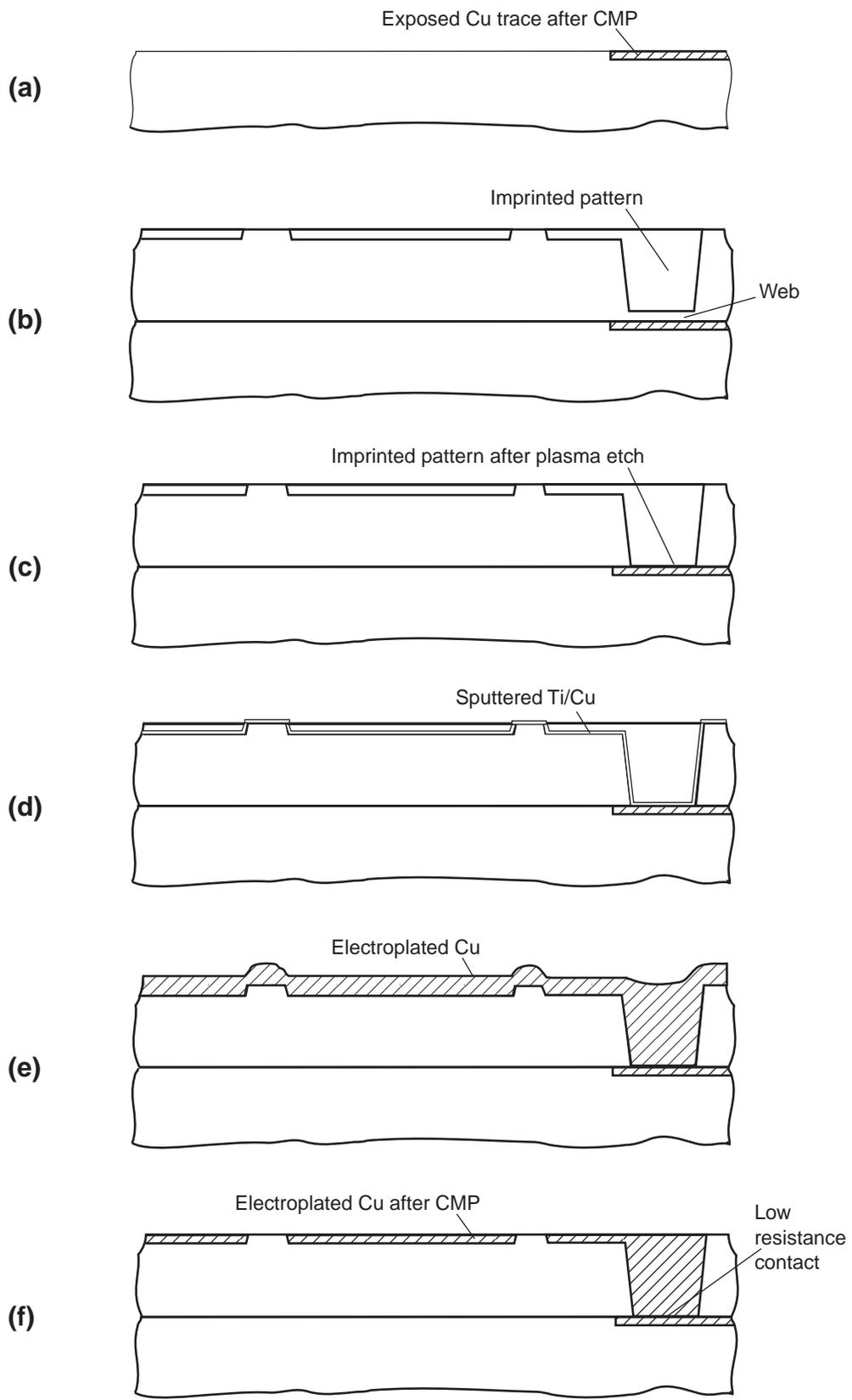
**Figure 7 - Summary of the Process Steps for Metallizing with Copper**
