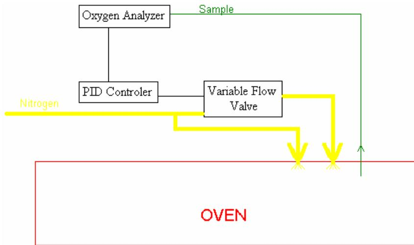
**Figure 1 – Example of Closed-loop Nitrogen Flow**
