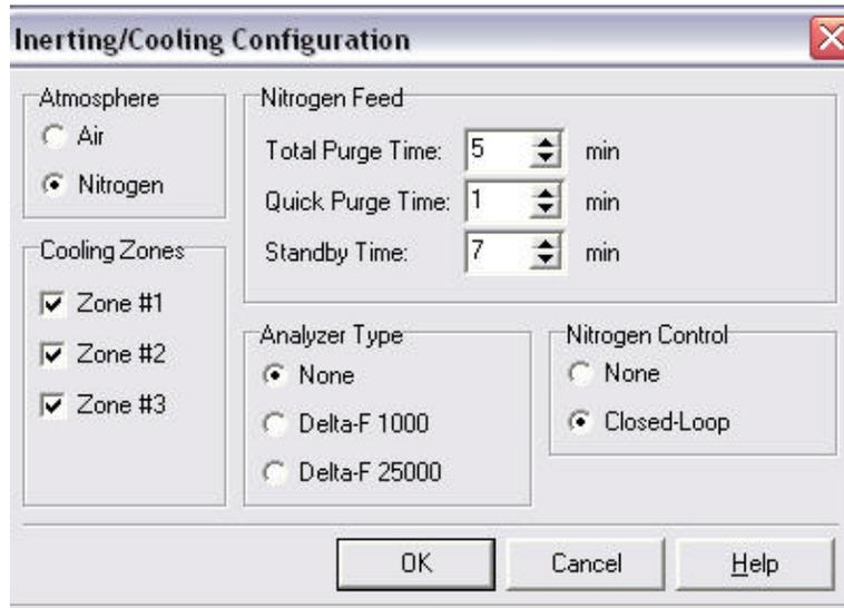
**Figure 2 – Nitrogen Flow Control Screen**
