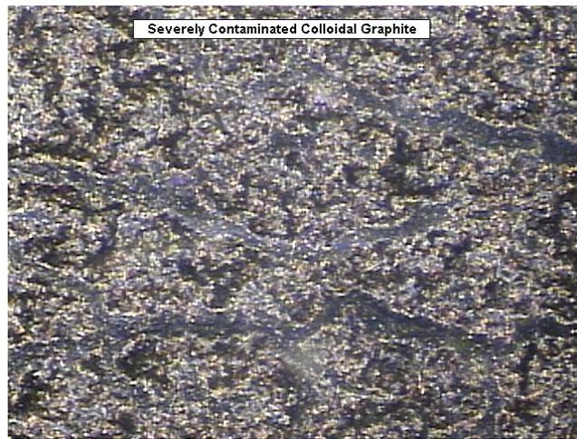
**Figure 5 - Magnified Glass Slide of a Contaminated Colloid**
