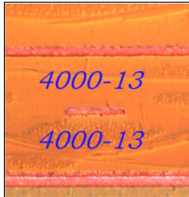
**Figure 10 - Cross Section N4000-13 Stripline**
