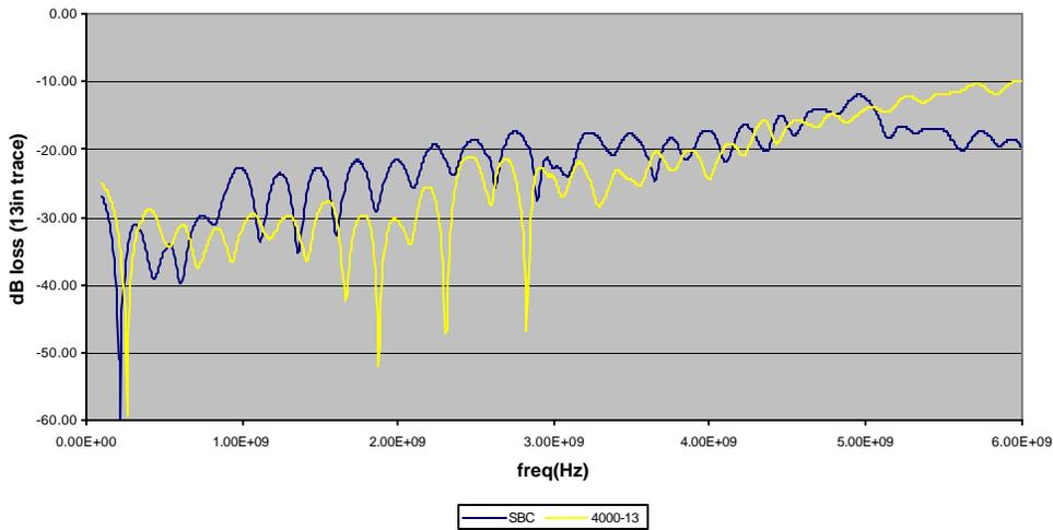
Figure15- Return loss of 2 materials through 6GHz
