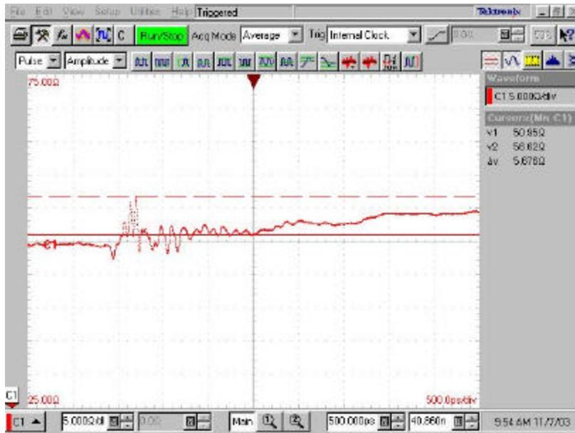
Figure13 - TDR of a Board Launch with a 5.6 ohm Discontinuity
