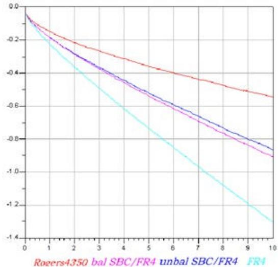
**Figure7 - Hybrid Stripline of Varying Materials and Thickness**
