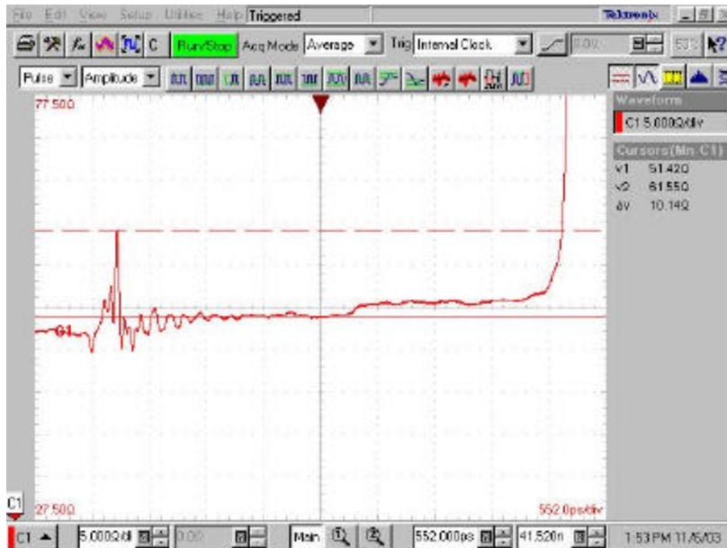
**Figure 11 - TDR of a Board Launch with Greater than 10 ohm Discontinuity**
