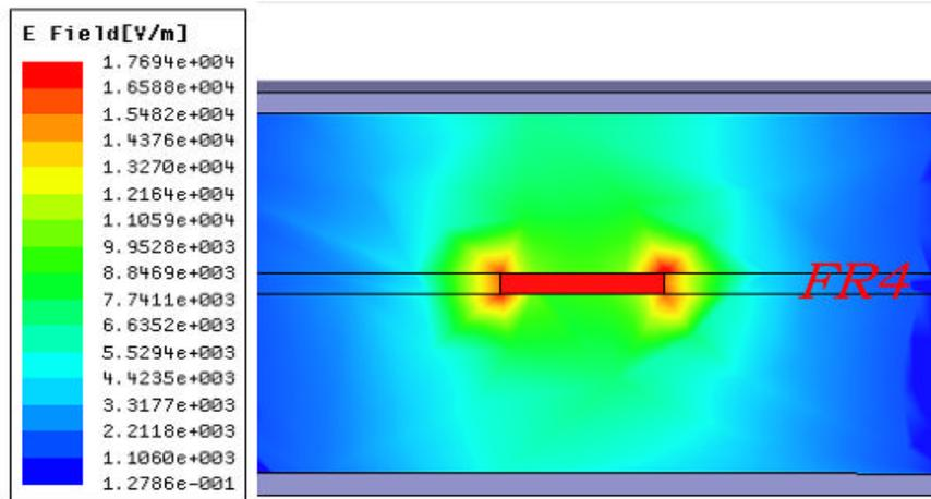
Figure2 - Magnitude of the Electric Field for an all FR4 Construction
