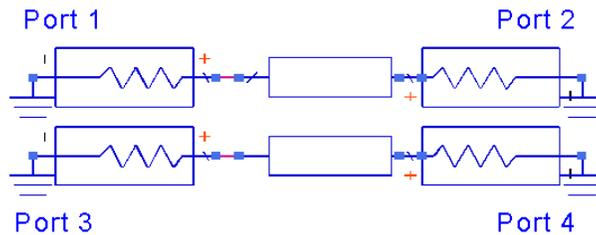
Figure 4 - Port Arrangement for Crosstalk Measurements
