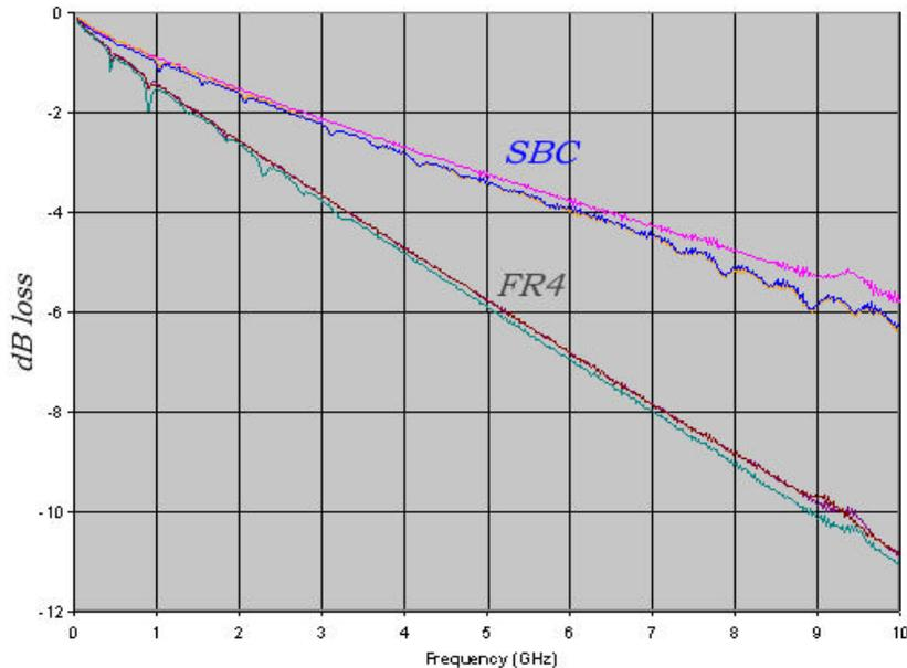
Figure 1 - Measured Loss of Several Microstrip Constructions
