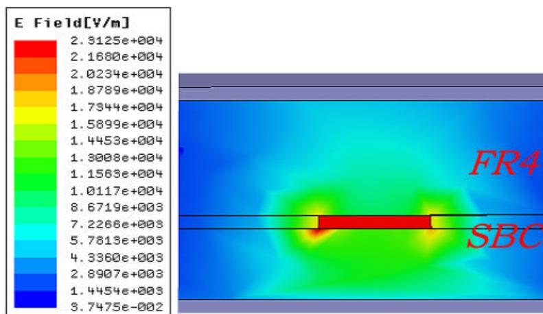
Figure3 - Magnitude of the Electric Field for a Hybrid FR4 -SBC Construction
