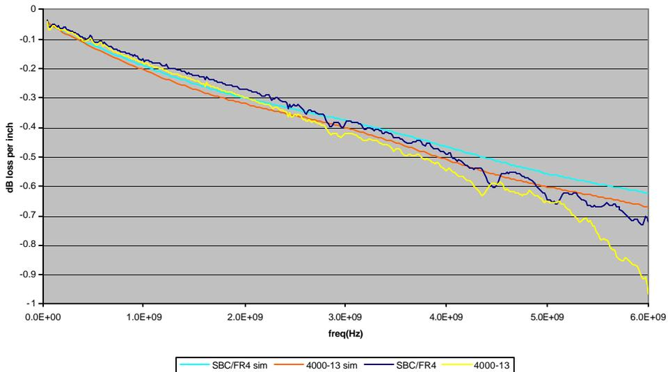
Figure16- comparison of simulated vs. measured data through 6GHz
