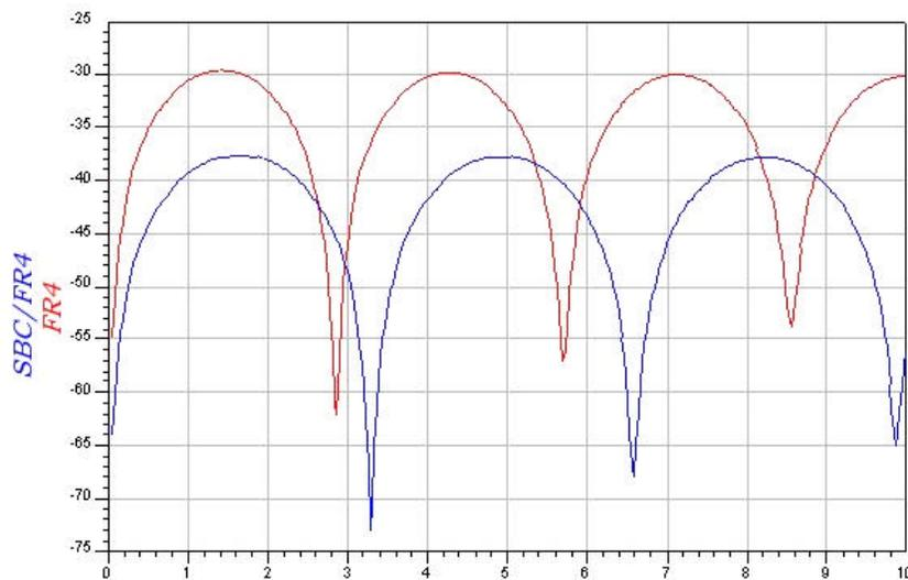
Figure 5 - NEXT of 6mil/6mil FR4 Stripline (red) vs. 3.4mil SBC/6mil FR4 Stripline (blue). Both Examples used a 10mil-space/4mil-trace Architecture
