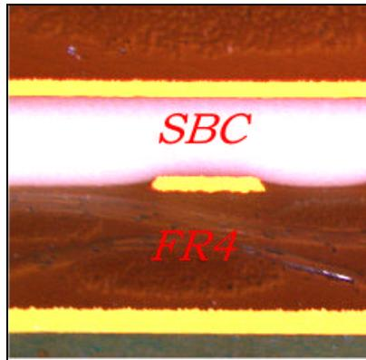
**Figure 9 - Cross Section SBC/FR4 Stripline**
