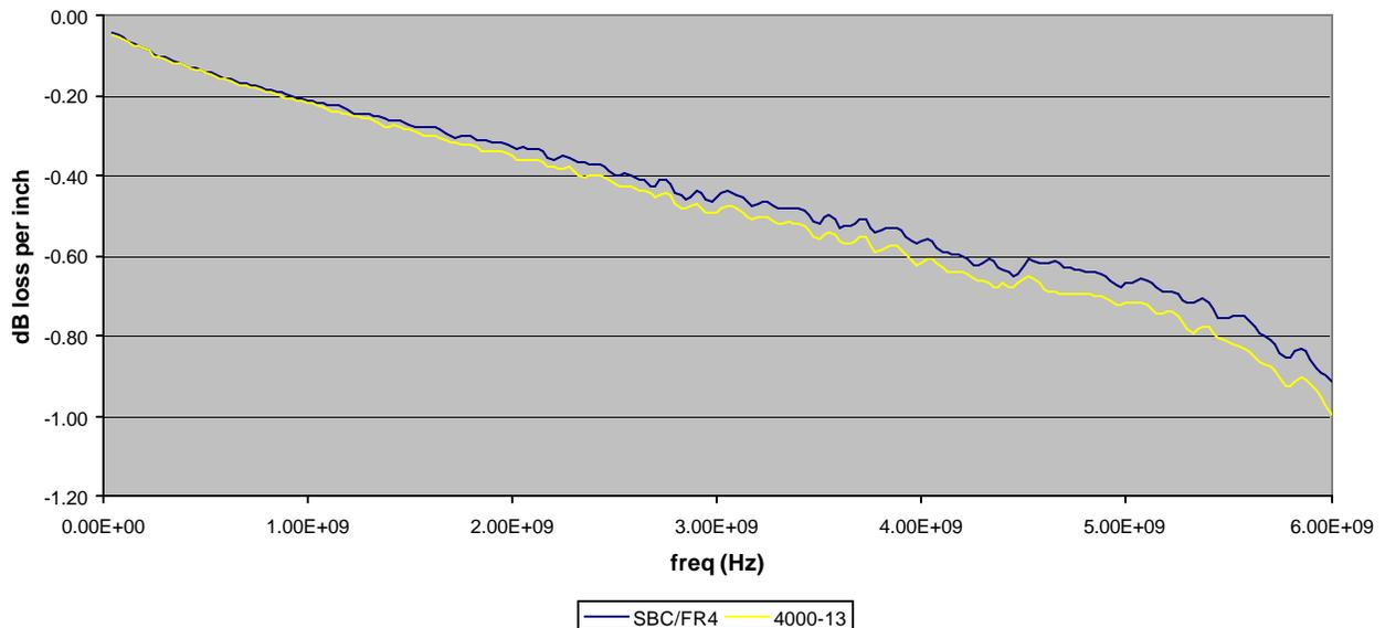
**Figure12 - Stripline with Board Launches of 10-20 ohm Discontinuities**
