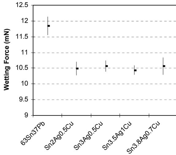
Figure 4 - Wetting Force of 63Sn37Pb and SnAgCu Solder Alloys determined at 245°C and 260°C, Respectively
