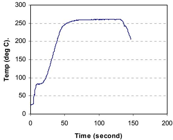
**Figure 1 - The Reflow Profile for the SnAgCu Pastes using a Vapor Phase Fluid with a Boiling Point of 260°C**
