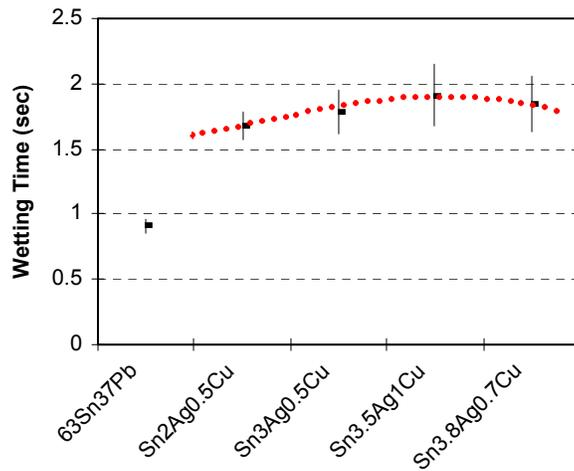
Figure 5 - Wetting Time of 63Sn37Pb and SnAgCu Solder Alloys determined at 245°C and 260°C, Respectively
