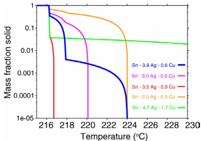
Figure 13 - Melting behavior of SnAgCu alloys<sup>10</sup>
