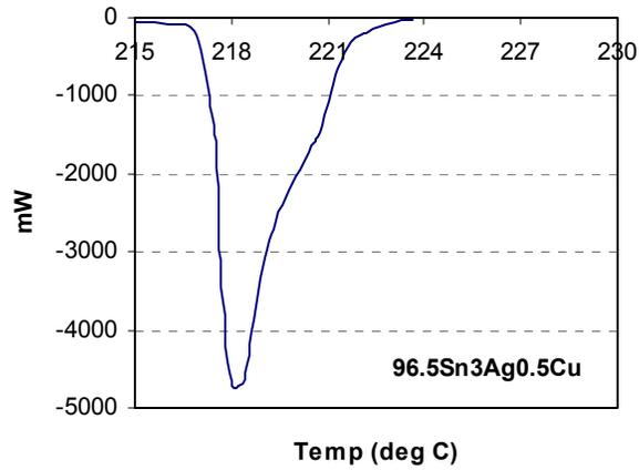
**Figure 9 - DSC Thermograph of 96.5Sn3Ag0.5Cu**
