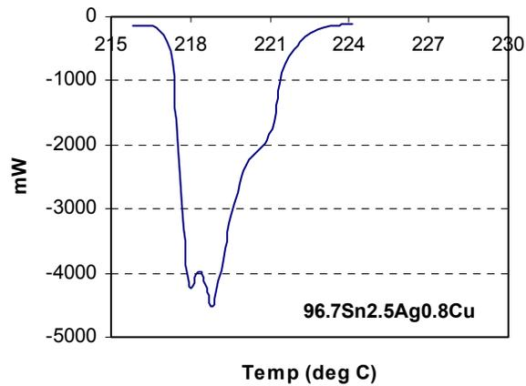
**Figure 10 - DSC Thermograph of 96.7Sn2.5Ag0.8Cu**
