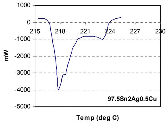
**Figure 11 - DSC Thermograph of 97.5Sn2Ag0.5Cu**
