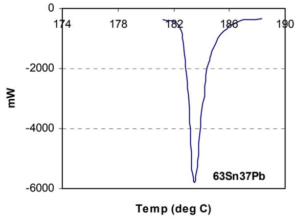
**Figure 6 DSC Thermograph of 63Sn37Pb Alloys**
