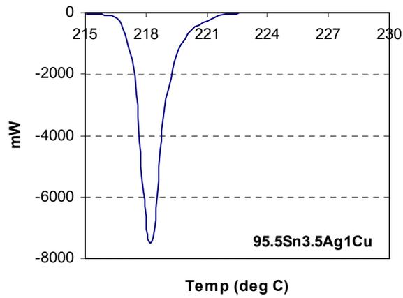
**Figure 8 - DSC Thermograph of 95.5Sn3.5Ag1Cu.**
