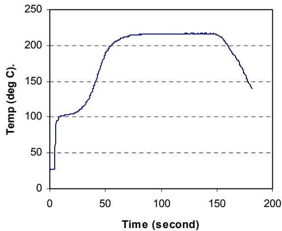
**Figure 2 - The Reflow Profile for the 63Sn37Pb Paste using a Vapor Phase Fluid with a Boiling Point of 215°C**
