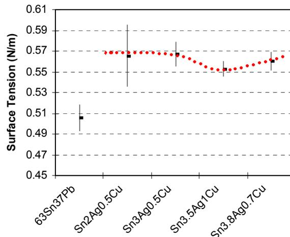
**Figure 12 - Surface Tension of 63Sn37Pb and SnAgCu Alloys determined at 245°C and 260°C, Respectively**
