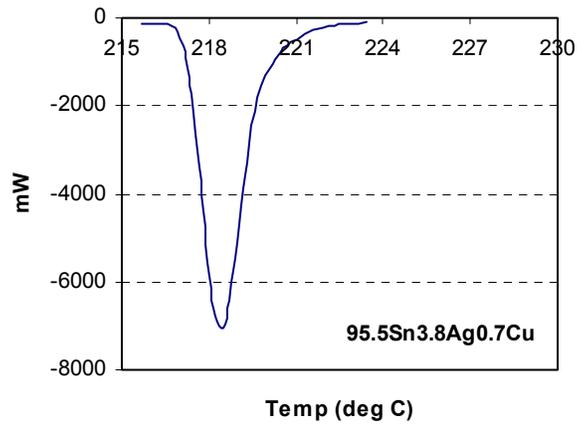
**Figure 7 - DSC Thermograph of 95.5Sn3.8Ag0.7Cu**
