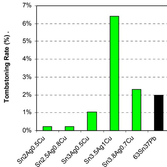
**Figure 3 - Tombstoning Rate of Solder Pastes with Vapor Phase Reflow Process - Here SnAgCu and SnPb Pastes were Reflowed at 260°C and 215°C, Respectively**
