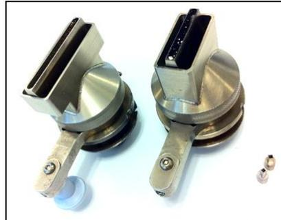
**Figure 15. Large Site Cleaning Nozzle (Zevac AG)**
