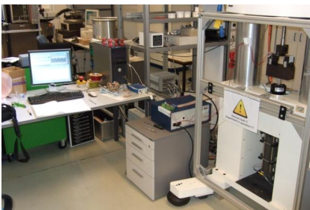
Fig. 7 - Board Level Cyclic Bend Test Set-Up
