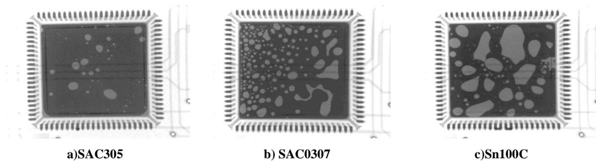
**Figure 15 – X Ray images of QFN88 components assembled with different lead-free alloy solder pastes. Low/no silver alloy solder pastes resulted in more voids and larger voids than SAC305 solder paste.**
