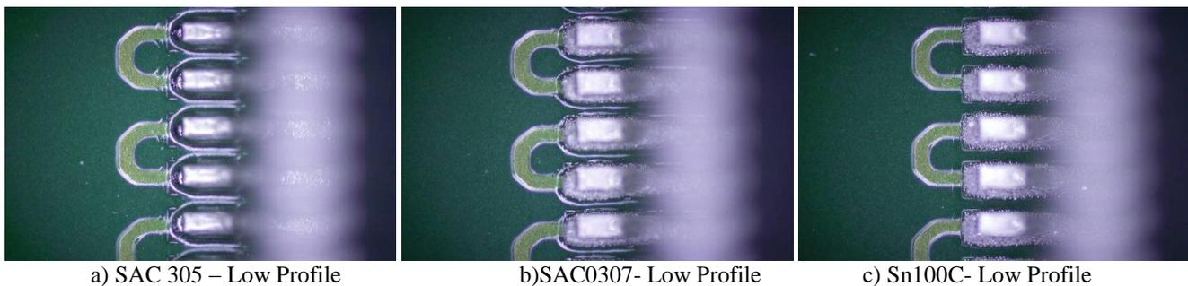
**Figure 16 – Visual images of solder joints reflowed with different lead-free alloys using low lead-free profile. 16a) Solder paste was melted for SAC305 alloy. 15b and 15c) Cold Solder was observed for SAC0307 and SN100C using a low lead-free profile.**
