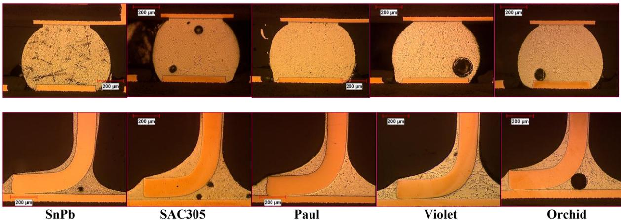
Figure 11: BGA325 and QFP240 structure, OSP, 100x
