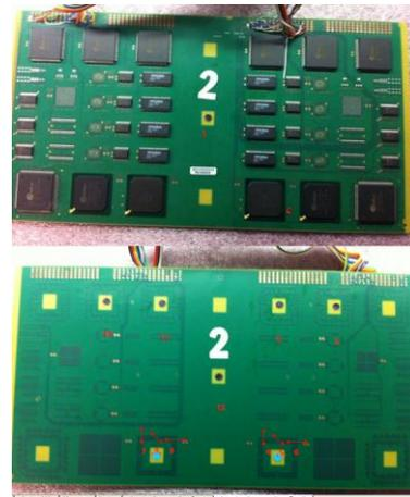
**Figure 8: Vibration Strain Gauge Location Scenario 2**
