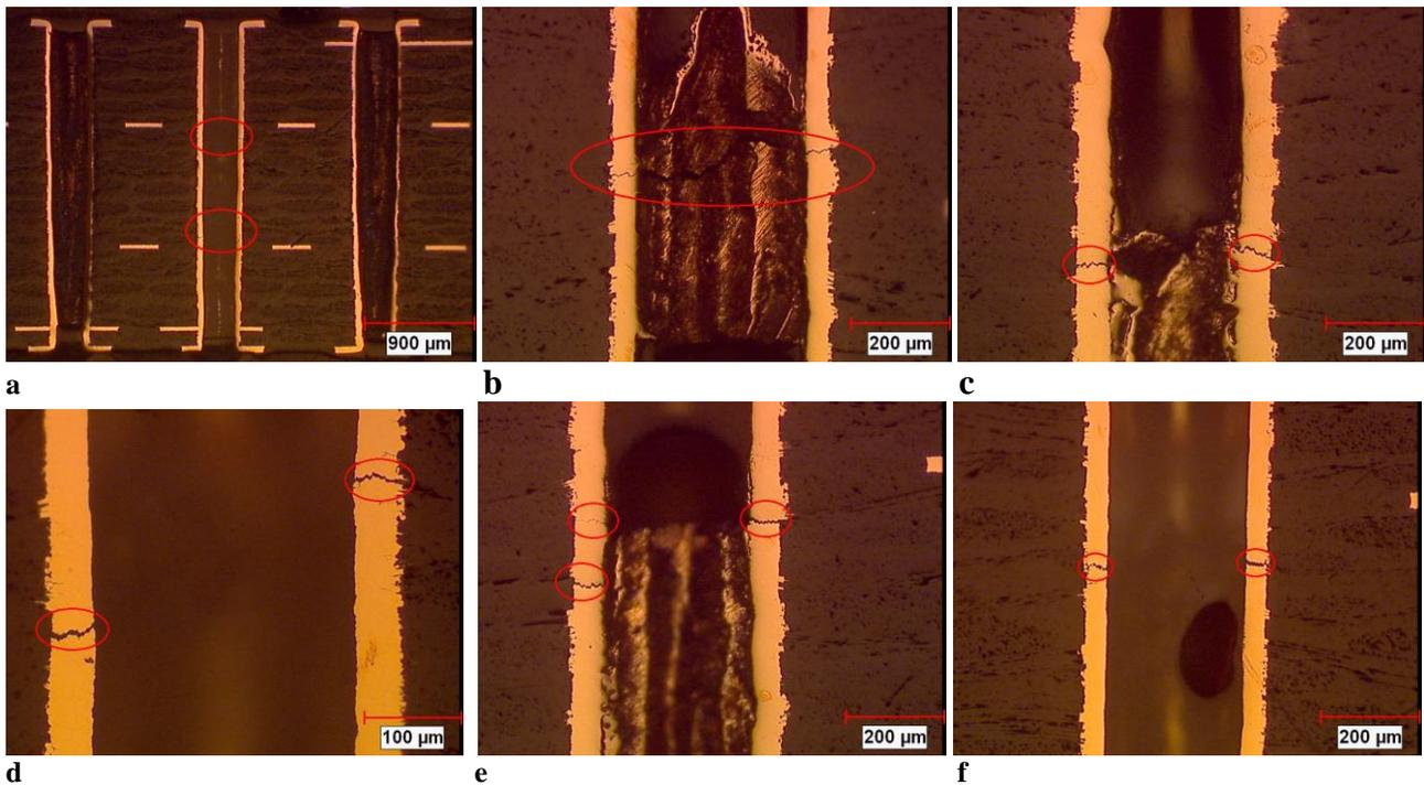
**Figure 21: Broken vias on 150°C TG boards with OSP finish after -55°C to 125°C cycling: a – Typical location; b – Circular shape; c - BGA352, Paul, 1067 cycles; d - Paul, 1067 cycles; e - C305, 853 cycles, 1255 cycles; e - Sn-Pb, 1257 cycles**
