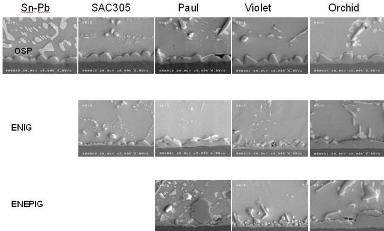
Figure 17: Intermetallic formation in QFP240, SEM, 5000x
