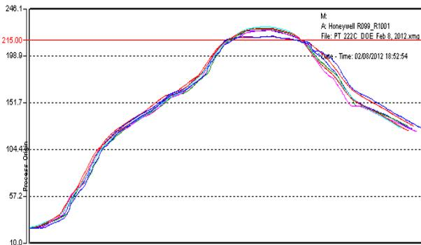
**Figure 2: Reflow Profile for 240°C**
