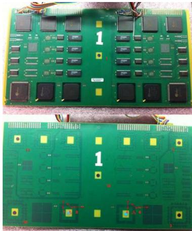
**Figure 7: Vibration Strain Gauge Location Scenario 1**
