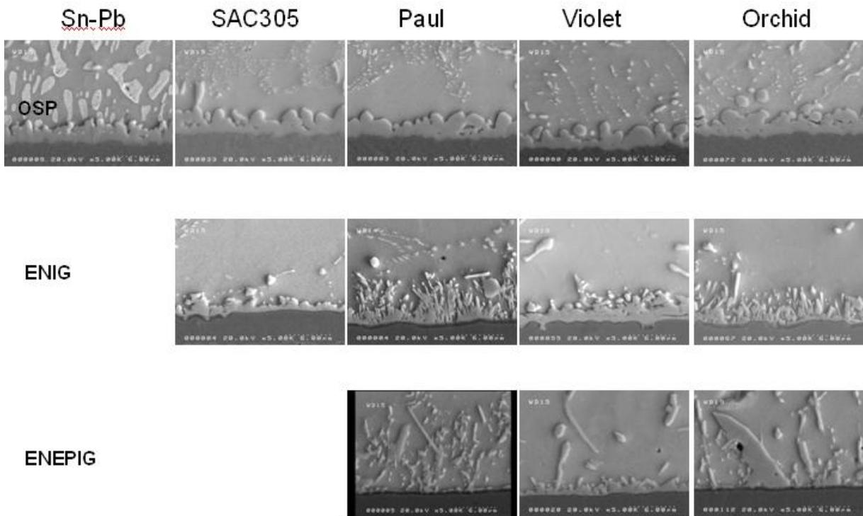
Figure 16: Intermetallic formation in BGA352, SEM, 5000x
