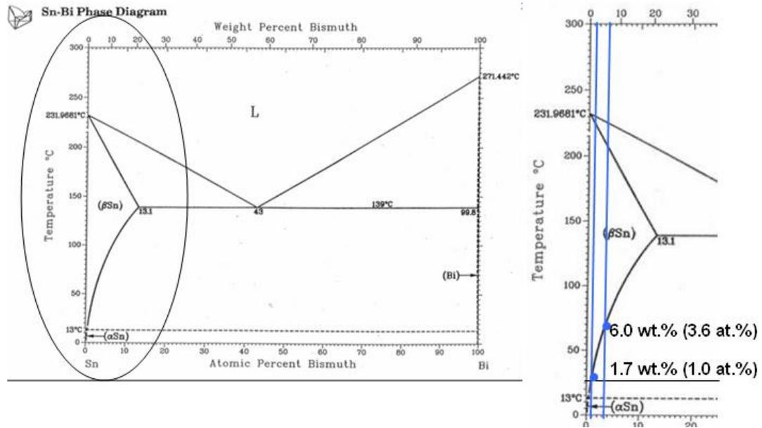
**Figure 13: Sn-Bi phase diagram showing Bi dissolution at different temperature**
