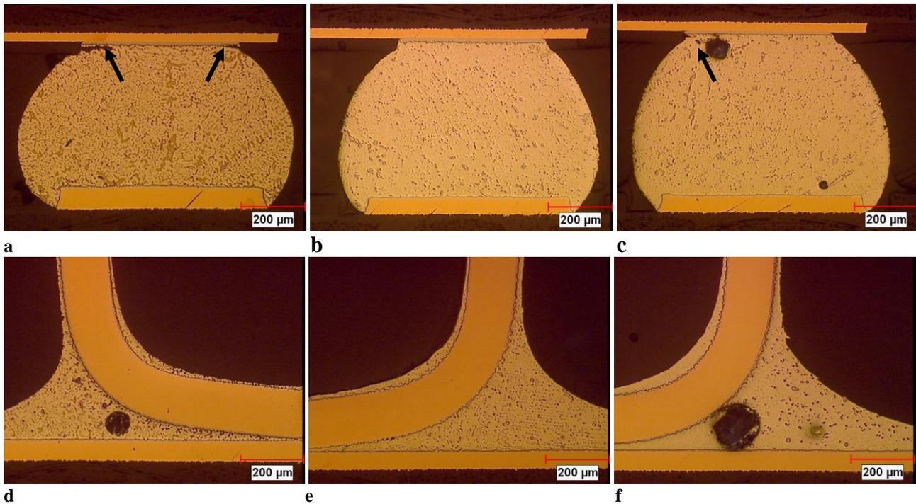
**Figure 20: Microstructure of solder joints formed on 150°C Tg boards with OSP finish after -55°C to 125°C cycling:**
