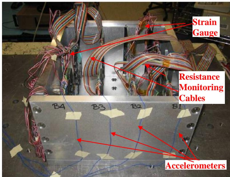
Figure 6: Vibration Fixture with Boards
