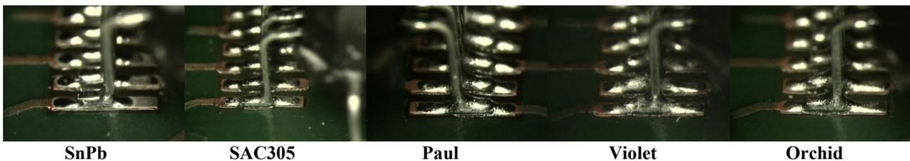
**Figure 10. Example of wetting on OSP, QFP240: A – SnPb; B – SAC305; C – OSP; D – Violet; E - Orchid**
