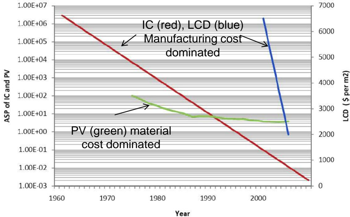
***Future cost reductions are much more likely for MEPV than wafered silicon PV since manufacturing costs are a much larger component of the module costs relative to material costs. (Typically manufacturing costs are driven down more rapidly than materials costs.)***
