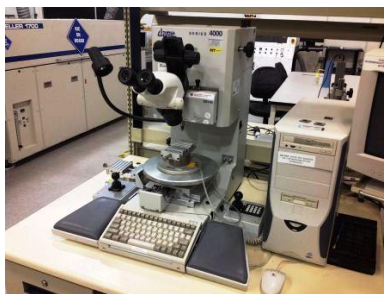
Figure 2A: Dage KE-2080 Shear Tester
