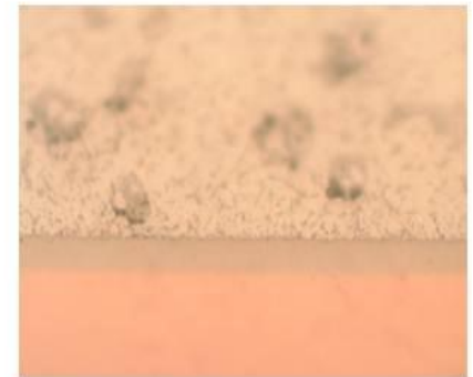
Original BGA: SAC405 Re-balled Alloy: Sn/Pb
