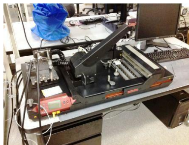
Figure 2B: Martin Expert 10.6 HV Rework Station
