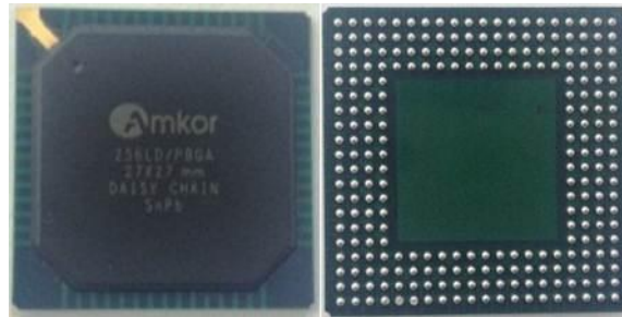
Figure 1: Amkor BGA used for Reballing and Shear Testing
