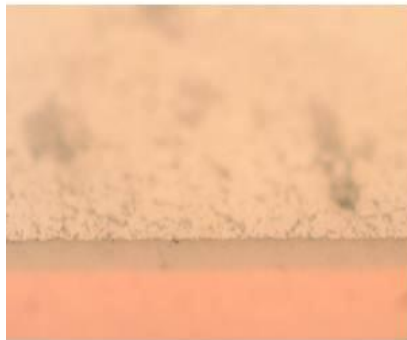
Original BGA: Sn/Pb Re-balled Alloy: Sn/Pb
