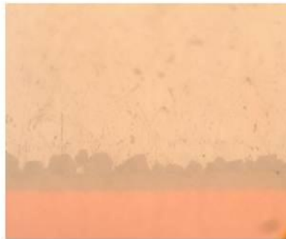
Original BGA: Sn/Pb Re-balled Alloy: SAC405
