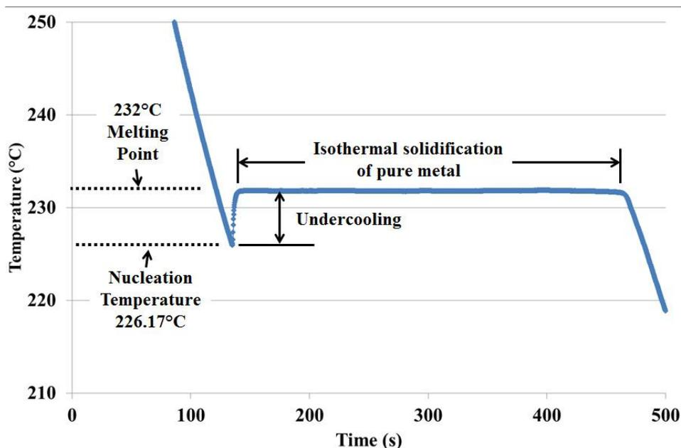
**Figure 1. Cooling curve for pure tin showing the undercooling required to trigger nucleation of solid.**
