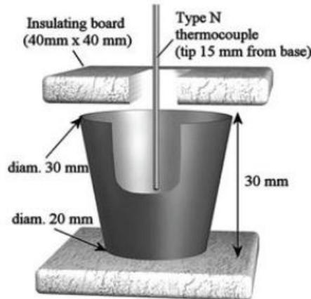
**Figure 3. Thermal analysis set up [ ]**
