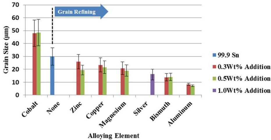
Figure 9. Effect of alloying addition on the recrystallized tin grain size. Results ranked by grain size with 0.3Wt% addition with results for pure tin and silver interpolated.
