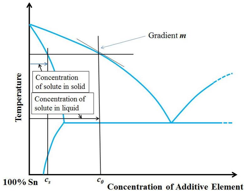
**Figure 2. Parameters used in the calculation of the Growth Restriction factor in non-equilibrium solidification.**
