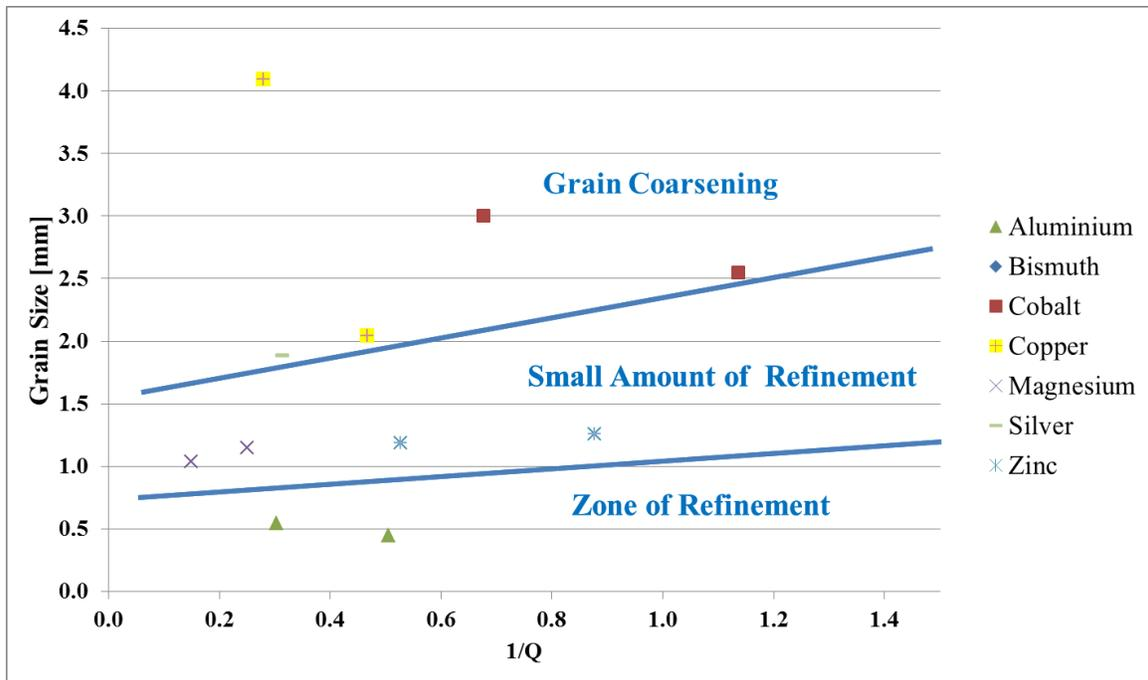
Figure 10. Relationship between the grain and the reciprocal of diffusion rate of solute atoms in the liquid at the solid liquid interface (the growth restriction factor).
