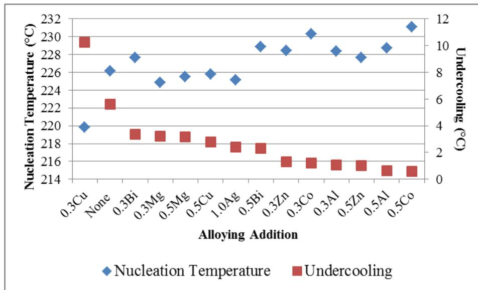
Figure 7. The effect of composition on nucleation temperature and undercooling with the results presented in order of decreasing undercooling
