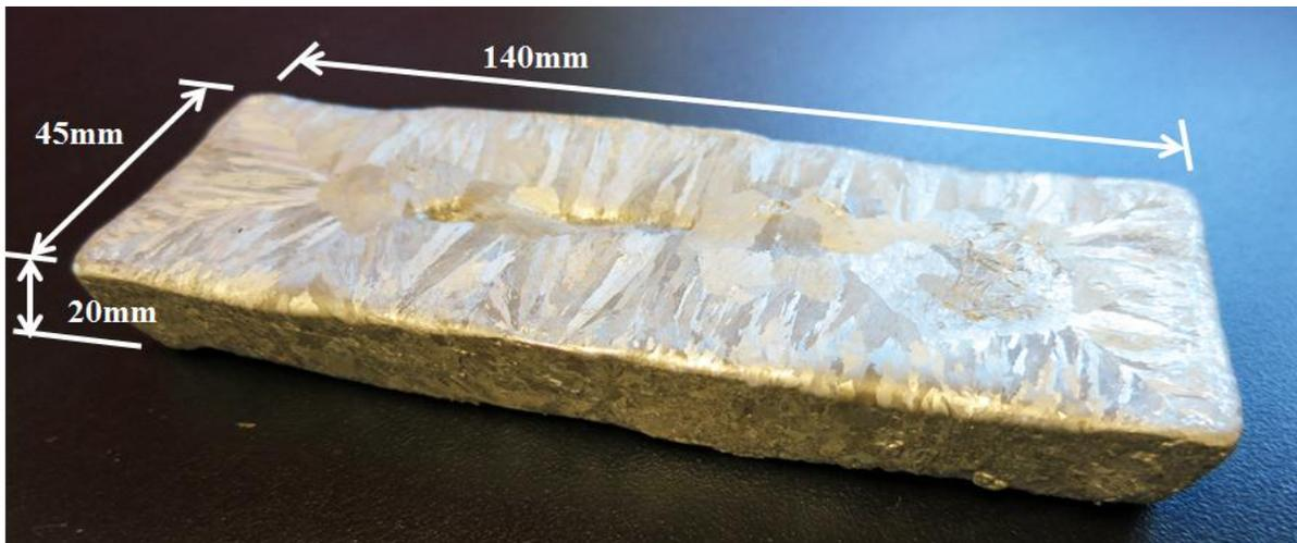
**Figure 4. Ingots cast for grain size determination.**
