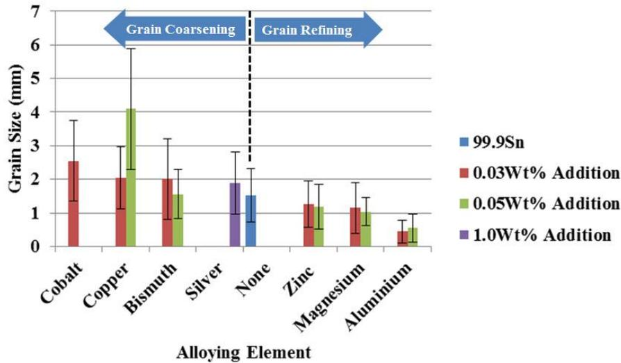
Figure 8. Effect of alloying addition on as-cast tin grain size.
