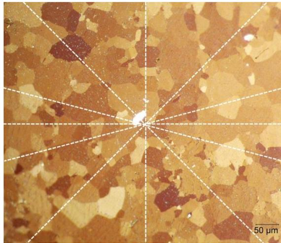
**Figure 6. Intercepts along which the recrystallized tin grain were counted in cross sections.**
