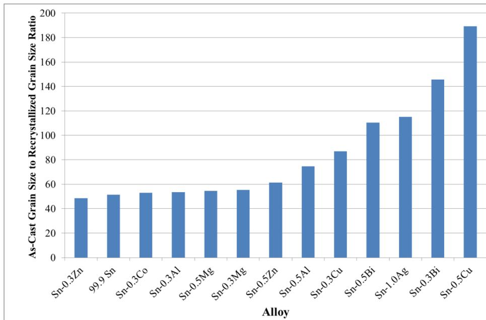
**Figure 11. Ratio of as-cast to recrystallized grain size as a function of alloy.**
