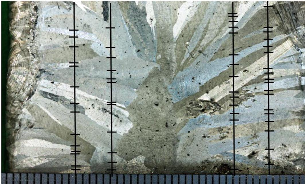
**Figure 5. Intercept counting method used to characterize the size of as-cast grains.**
