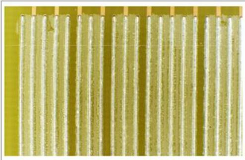
**Figure 5.** Paste 55 Post T Shock Delamination
