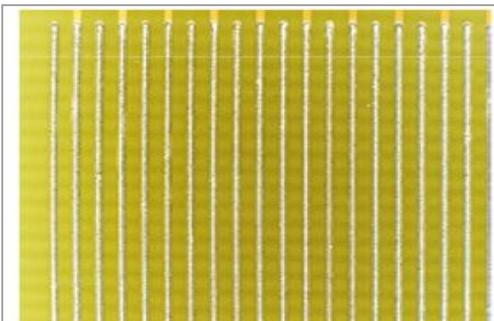
**Figure 7.** Paste 16 Post T Shock/No defects
