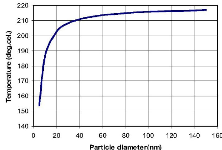
Theoretical plot of the melting point due to nanosize effect as function of particle size for Sn-4.0Ag-0.5Cu alloy.
