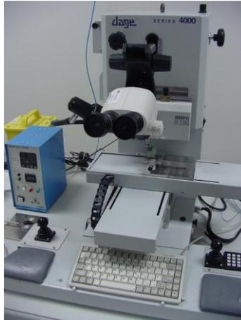
Figure 11: Dage 4000 slow speed bond tester
