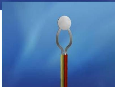
**Figure 2. Flattened TC bead located directly underneath the BGA**
