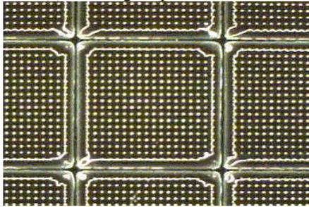
(b) coating on area array wafer
