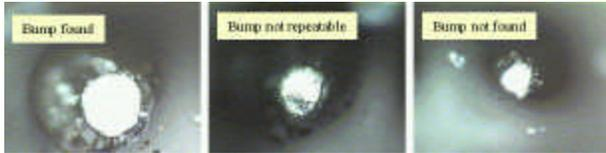
**Figure 5 - Bumps on Coated Die as Inspected by the Universal Vision System**
