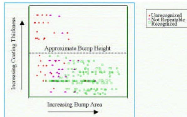
**Figure 7 - Bump Area Versus Coating Thickness**
