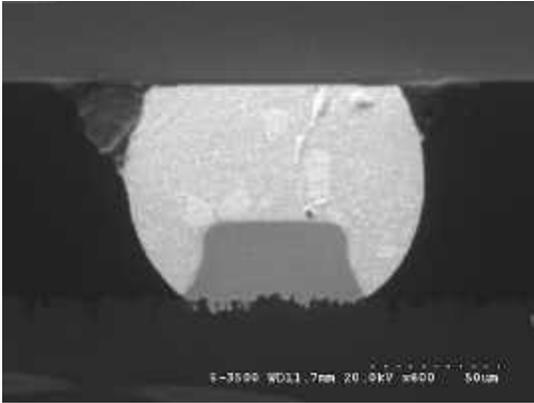
(a) Solder joint formed after storing chip for 6 months
