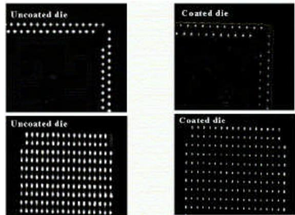
**Figure 4 - Vision system images of perimeter I/O chip (top) and area array chip (bottom)**
