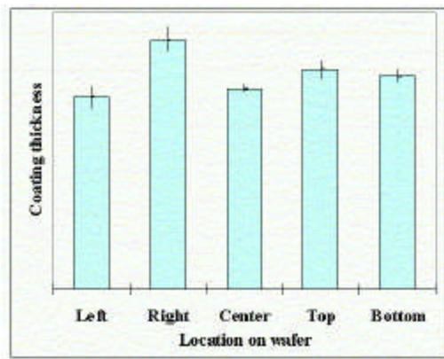
(a) thickness data for perimeter I/O wafer
