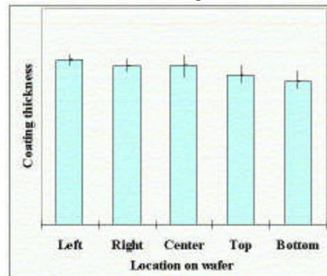
(b) thickness data for area array wafer
