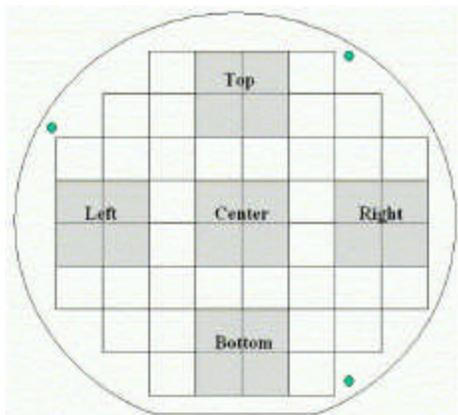
(a) 12-mil pitch perimeter I/O wafer layout
