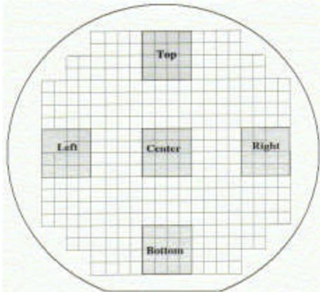
(b) 10-mil pitch area array wafer layout
