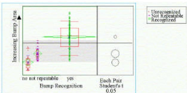
**Figure 6 - Bump Recognition Versus area Measurements**
