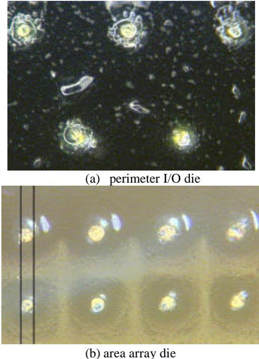
**Figure 8 - Appearance of Chip Tacked to Glass Slide**
