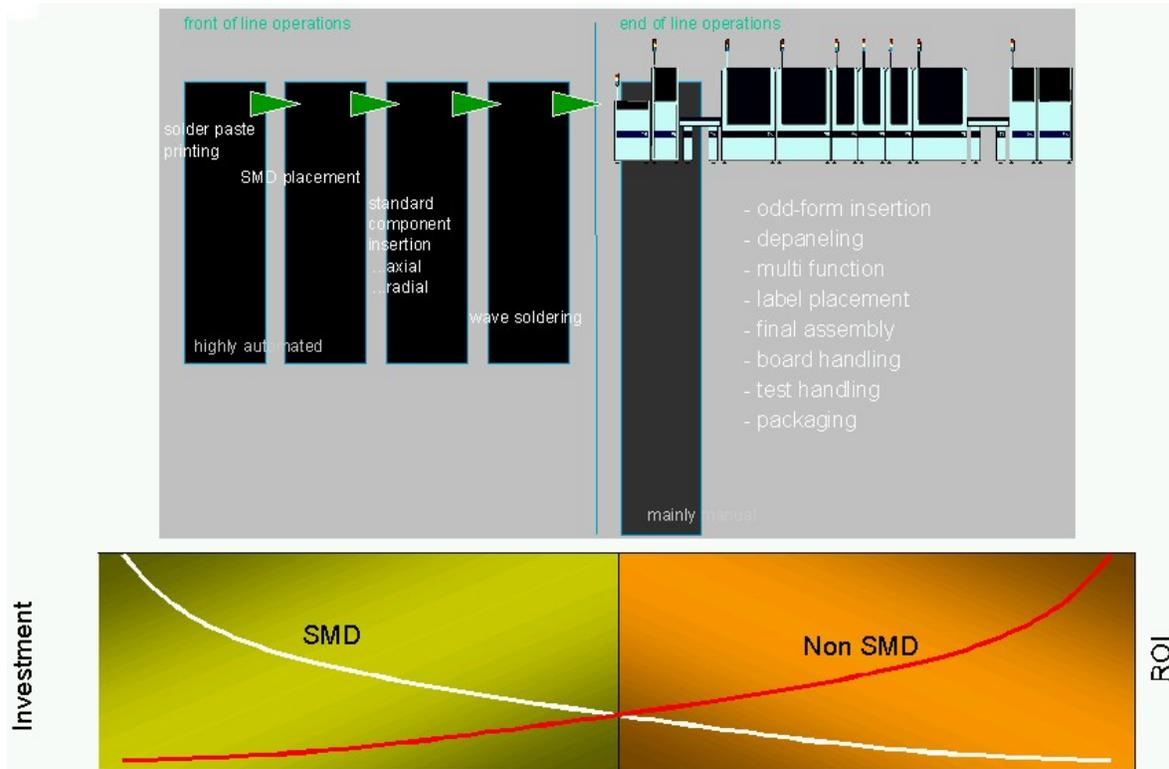
**Figure 3 - The Relationship Between Payback/ROI in the SMT and EOL Situation Can be Best Described this Way: Millions of Dollars in SMT Equipment Buys You a Line Similar if not Identical to Many Others - It Pays Back at a Rate Well Described by Industry Norms - A Significantly Smaller Investment in EOL Automation Allows New Operational Practices to be Realized that Differentiate and Drive High Levels of Return**
