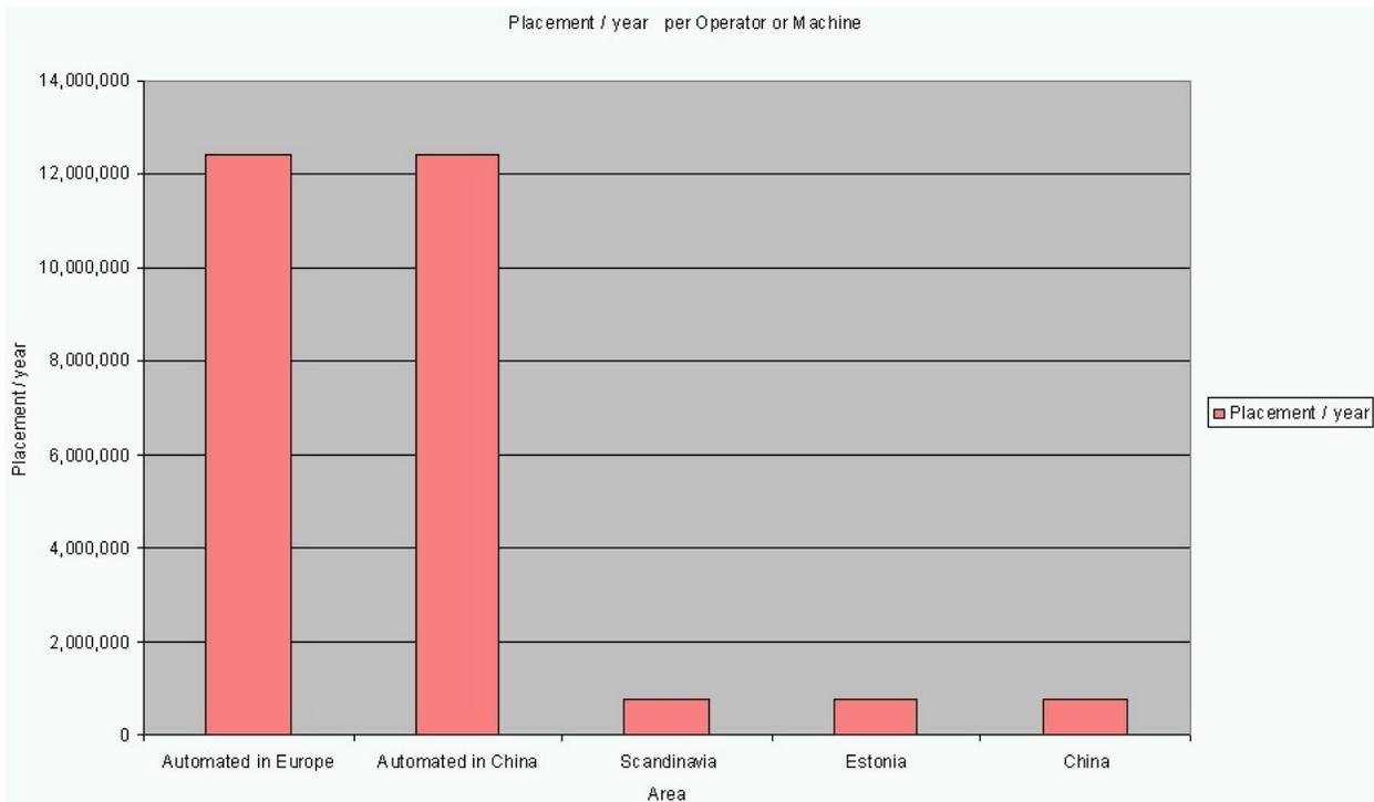
**Figure 5 - Parts Placed Per Year by an Operator vs. AUTOMATED SYSTEMS is a Fraction, Further Illustrating the Impact of Fast Ramp Up or Down and the Impact that it has on a Companies Performance and Cost**
