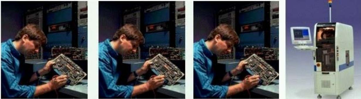
**Figure 2 - A Typical EOL Automation System Today Consists of One or More Cells of 0.5 Meters each in Length - Typically each Cell can Provide the Output Equal to 3 Operators**
