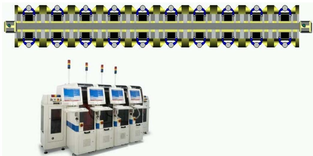
**Figure 4 - Familiar Line Above Measuring 16m in Length was Replaced with a Machine Solution 3.5M in Length that Required 1 Operator Per Shift**
