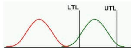
**Figure 2 - The Tolerance Limits can be Defined More Optimally to Fail Fewer Good Solder Joints (green=good}right : red=bad}left )**
