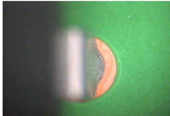
**Figure 4 - Category 2: Solder Has Filled The Hole Completely But The Topside Pad is Not Fully Wetted**
