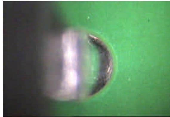
**Figure 3 – Category 1: Solder Has Filled The Hole Completely and The Topside Pad is Fully Wetted**
