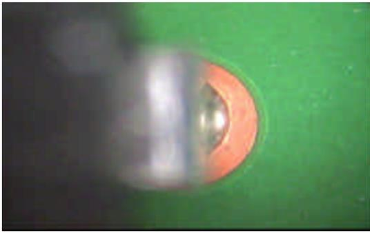
**Figure 5 – Category 3: Solder Has Not Completely Filled The Hole and Topside Pad is Not Wetted**
