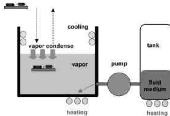
**Figure 3 - Vapor Phase Soldering with Unsaturated Vapor Atmosphere<sup>3</sup>**
