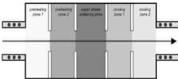
**Figure 7 - Structure of a True Inline Condensation Soldering Machine**
