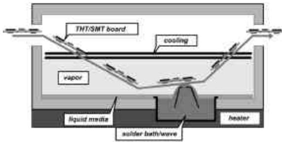
**Figure 4 - Combination of Reflow Soldering and Wave Soldering in a Vapor Phase<sup>4</sup>**
