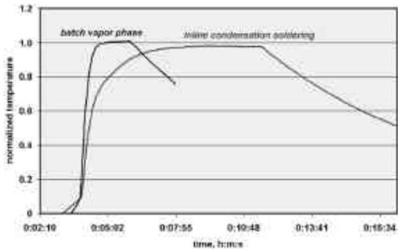
**Figure 12 - Comparison of Temperature Rise for a Standard Batch Vapor Phase and the "Inline" Condensation Machine**
