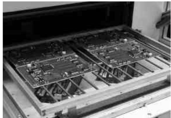
**Figure 6 - Tandem Carrier with Printed Circuit Boards<sup>4</sup>**
