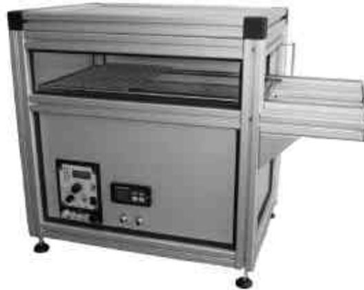
**Figure 8 - Laboratory Machine for Experimental Investigation of Inline Condensation Soldering**
