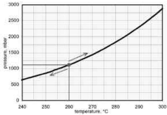
**Figure 9 - Boiling/Condensation Temperature of a 260°C Media Depending on Vapor Pressure**
