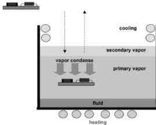
**Figure 2 - Modified Vapor Phase Process with Two Different Vapor Covers<sup>2</sup>**
