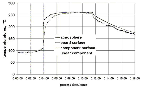
**Figure 11 - Measured Temperature Profiles for Condensation Soldering in the "Inline" Machine**
