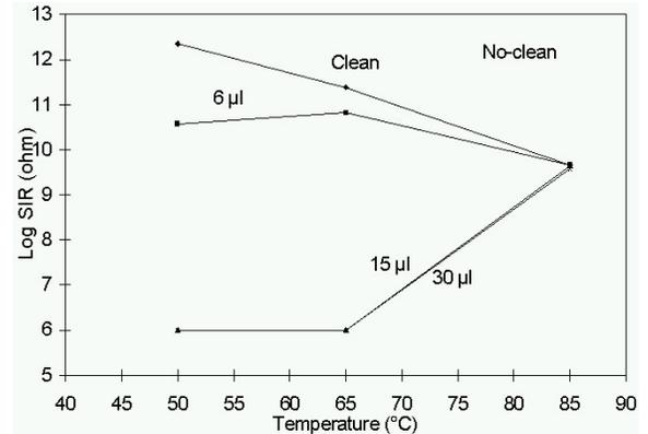
Figure 12 - Below 65°C, with 15 & 30 µl Applied, the No-Clean Flux Gives a Very Low SIR Reading
