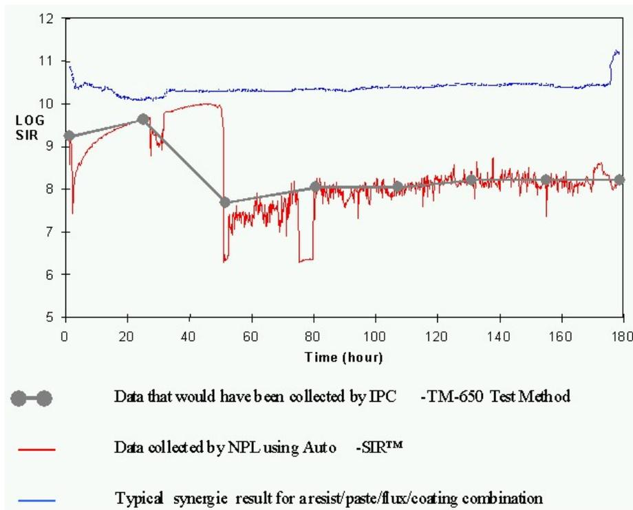
**Figure 13 - Current Standards will only Detect Dendritic Growths if they Occur at Exactly the Same Time as the Measurement**
