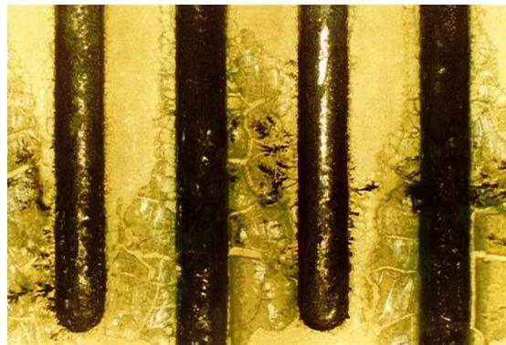
**Figure 2 – Field Failures and SIR Test Failures can be Dramatic**
