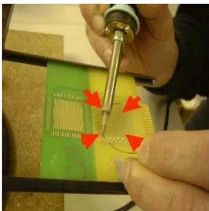
**Figure 7 – Solder Rework to Prepare the Sample**
