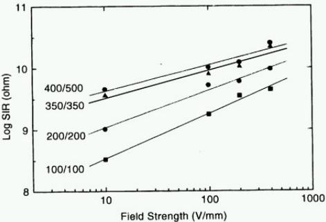
**Figure 15 - Effect of Field Strength on SIR Increases as the Pitch of the Coupon Decreases**
