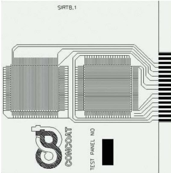
**Figure 3 – Test Substrate – Surface Mount SIR Coupon**
