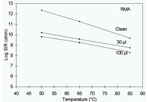
Figure 11 - Effect of High Temperature for Traditional RMA Fluxes is to Reduce SIR
