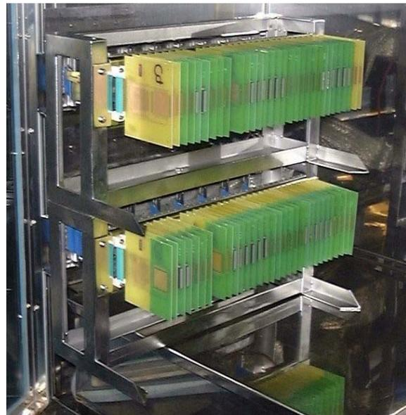
**Figure 8 - Test Rack Shown in Environmental Chamber**
