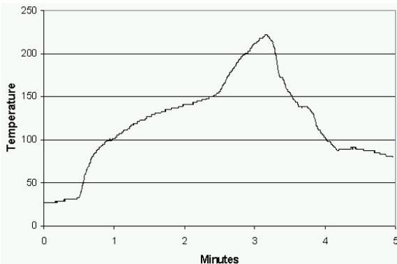
**Figure 6 - Reflow Temperature Profile**
