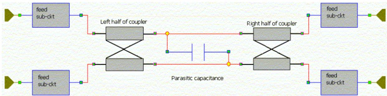
**Figure 3 – Electrical Model of Bi-Directional Coupler A**
