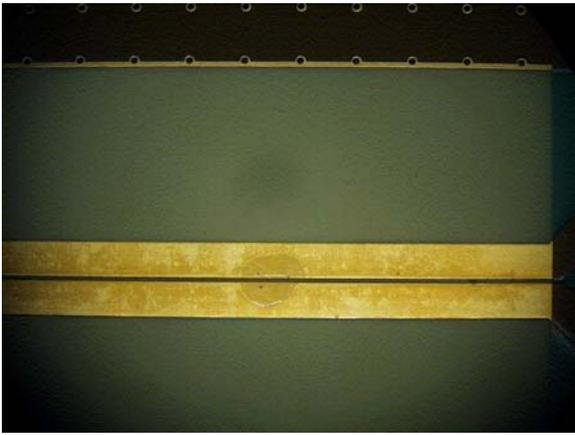
**Figure 6 – Darker Areas on the Traces Around the Central Dispensed Dot Occurs During Aging**
