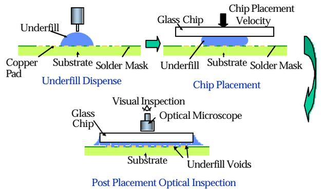
**Figure 5 - Chip Attach Test Process and Response Observation**
