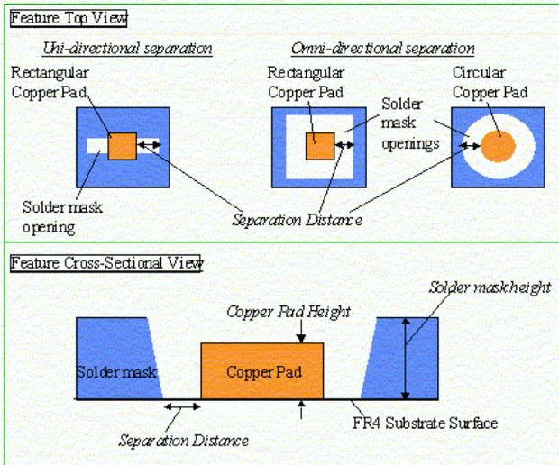
**Figure 2 - Schematics of Substrate Design Factors Varied in Experimentation**
