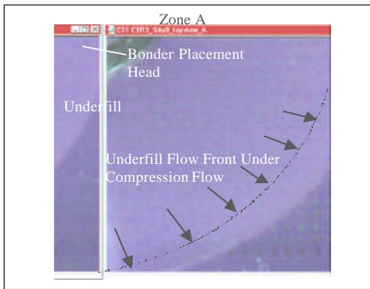
**Figure 7 - Placement Process of Glass Chip on Test Site (0.283 seconds after Figure 6). Underfill Compressed Under Chip Inducing Flow Front Over Pads**
