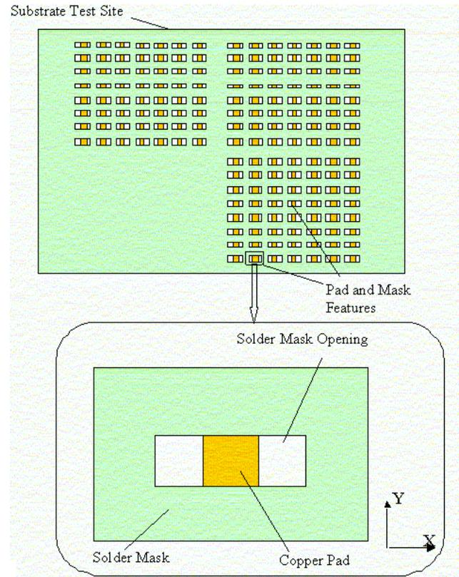
**Figure 1 - Typical Substrate Test Site and Feature**
