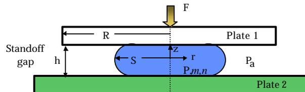
**Figure 11 - Compression Flow between Equivalent Circular Parallel Plates**
