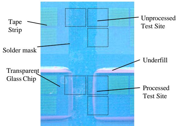
**Figure 4 - Assembled Test Substrate Site with Underfill Dispensed and Glass Chips Placed**
