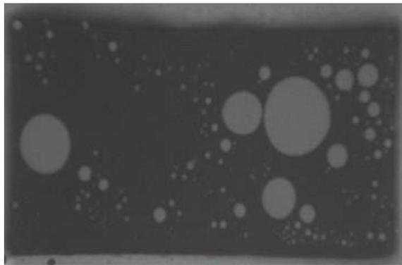
**Figure 4 Example of X-ray Picture of Reflowed Sample**
