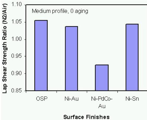
**Figure 12 - Sensitivity of Lap Shear Strength Toward Reflow Atmosphere for System with Medium Profile and Aging 0 Treatment**
