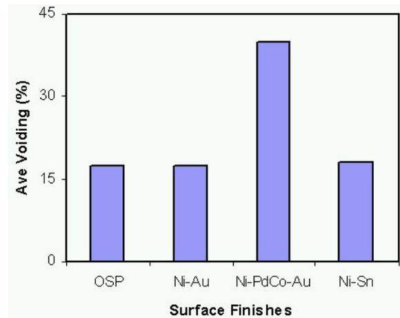
**Figure 7 - Effect of Surface Finish on Voiding**
