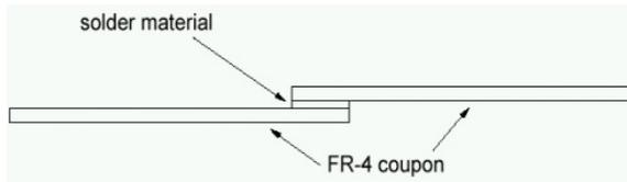
**Figure 3 Schematic of Side View of Lap Shear Sample Layout**
