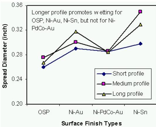
Figure 8 - Effect of Profile Length on Wetting
