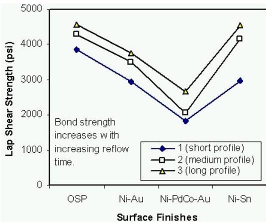
Figure 9 - Effect of Profile Length on Bond Strength
