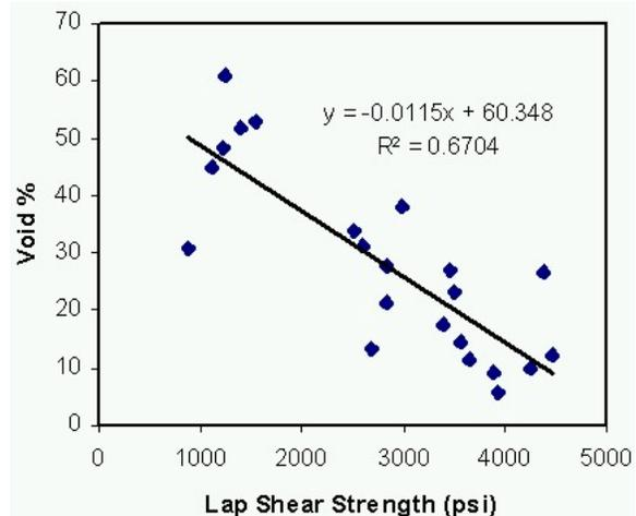
Figure 19 - Relation between void content and lap shear strength for SnBiAg system.
