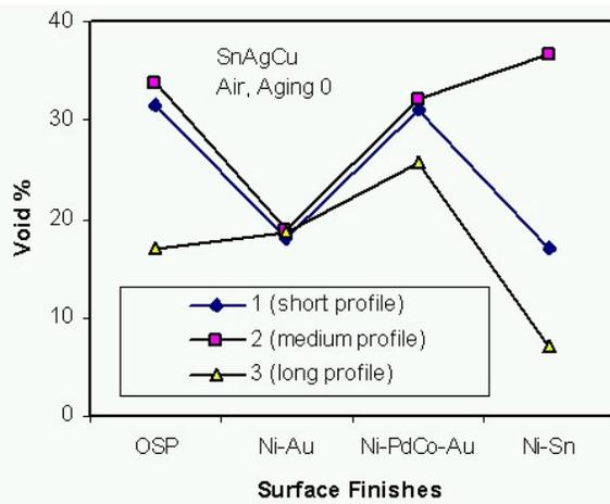
Figure 10 - Effect of Profile Length on Voiding for SnAgCu System with Aging 0 and Air Reflow Atmosphere
