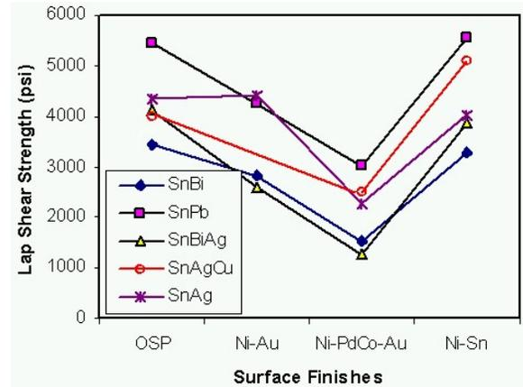
**Figure 15 - Effect of Solder Alloys on Lap Shear Strength**
