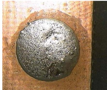
**Figure 2 - Example of Solder Circle after Reflow**
