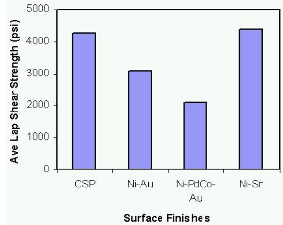
**Figure 6 - Effect of Surface Finish on Bond Strength**
