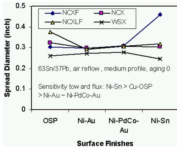
Figure 18 - Effect of Flux Chemistry on Wetting
