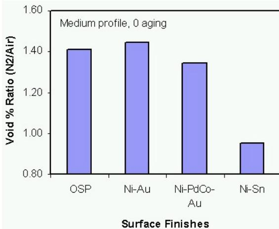
**Figure 13 - Effect of Reflow Atmosphere on Voiding for a System with Medium Profile and Aging 0 Treatment**
