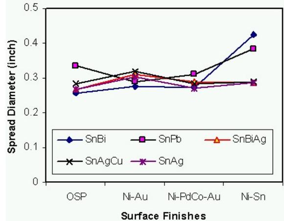
**Figure - 14 Effect of Solder Alloy on Wetting**
