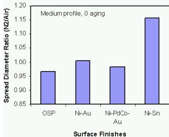
Figure 11 - Effect of Reflow Atmosphere on Wetting - A Ratio Value Greater than One Indicates a Positive Effect of Nitrogen.
