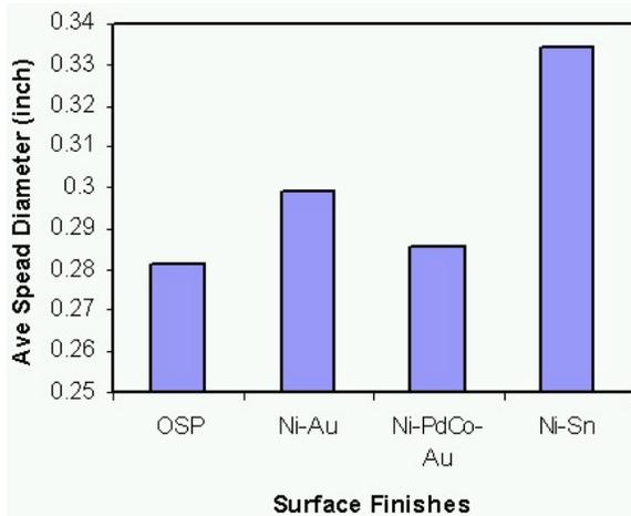
**Figure 5 Effect of Surface Finish on Wetting**
