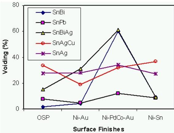
Figure 16 - Effect of Solder Alloys on Voiding
