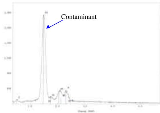
**Figure 5 - EDX Spectrum showing that Al is a Source of Contaminations**
