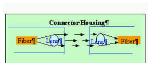
Figure 2 - Lensed Connector Configuration
