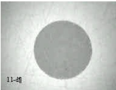
**Figure 11 - Scratches on Optical Connector**
