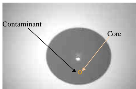
**Figure 9 - Contaminant on Core and Cladding Total Contamination Area is about 44 $\mu\text{m}^2$**
