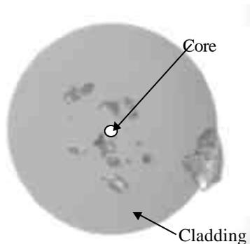
**Figure 8 - Contaminants on Cladding and Close to Core Total Contamination Area is about 1120  $\mu\text{m}^2$**
