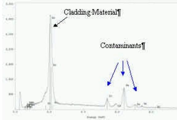
**Figure 4 - EDX Spectrum of Optical Connector’s Contaminants Showing Contaminants (Cr, Fe, Ni) from Connector Adapter**
