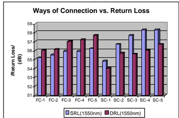
**Figure 13 - Return Loss Measurements Using Different Connection Means. SRL = Return Loss Using Same Type Connector Adapter. DRL = Return Loss Using Different Type Connector Adapter**
