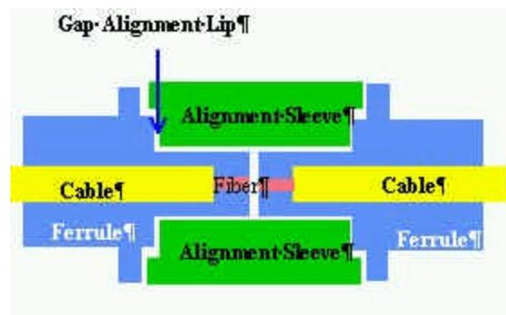
Figure 1 - Straight Sleeve Connector Design
