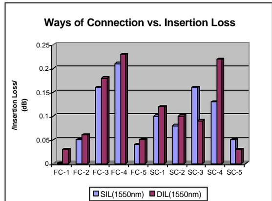
**Figure 12 - Insertion Loss Measurements Using Different Connection Means. SIL = Insertion Loss Using Same Type Connector Adapter. DIL=Insertion Loss Using Different Type Connector Adapter**
