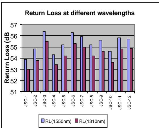
Figure 15 - Return Loss of SC Fiber Optic Connectors at Different Wavelengths
