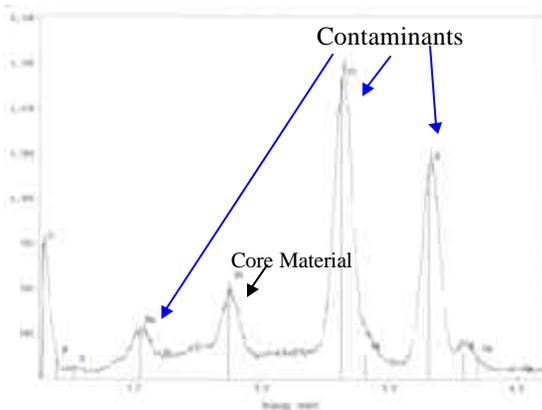
**Figure 3 - EDX Spectrum of a Contaminated Connector Showing “Human” Contamination**
