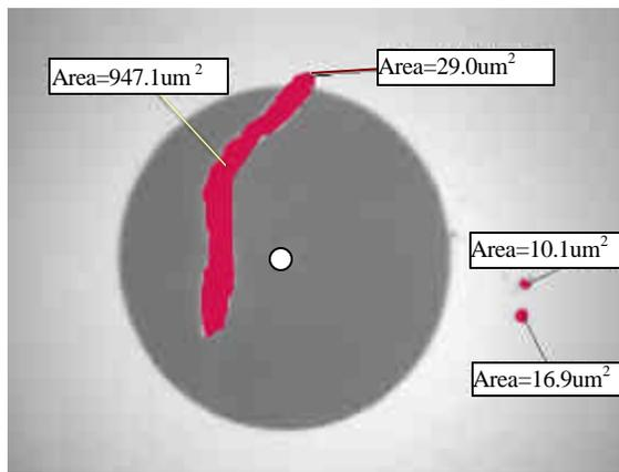
**Figure 7 - Contaminations on Cladding-A loss of about 0.04 dB was seen (total contamination area is about 1003.8  $\mu\text{m}^2$ )**
