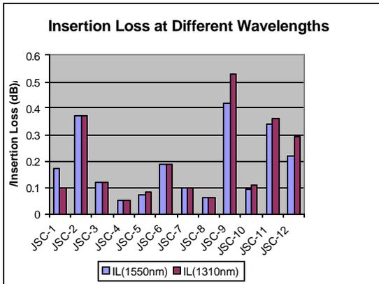
Figure 14 - Insertion Losses of Optical Connectors at Different Wavelengths
