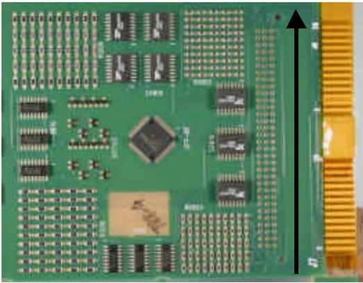
**Figure 1 - Arrangement of SMT Components for One Circuit on the Bottom of the Test Vehicle for Wave Soldering Arrow Shows Feed Direction**
