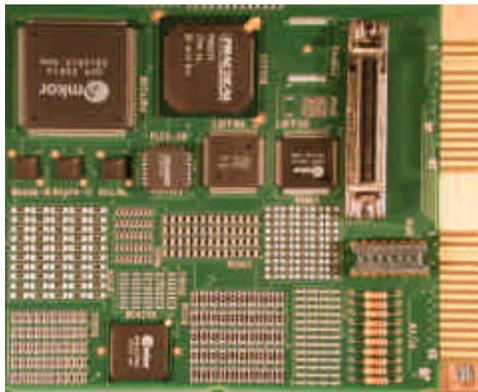
**Figure 2 - Arrangement of SMT and TH Components for One Circuit on the Top of the Test Vehicle for Reflow Soldering**
