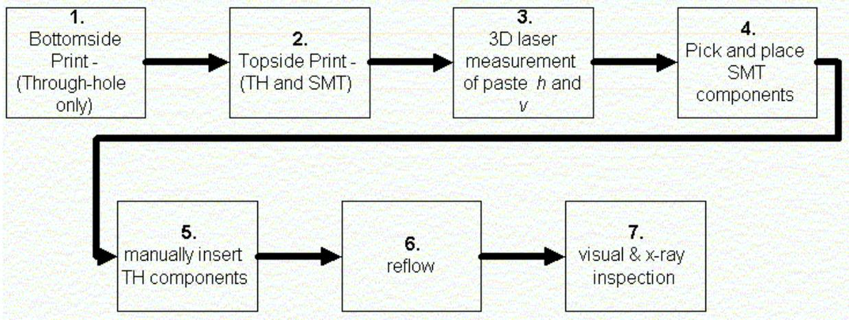
**Figure 4 - Process Flow for Pb-Free Paste-Reflow Assembly Process**
