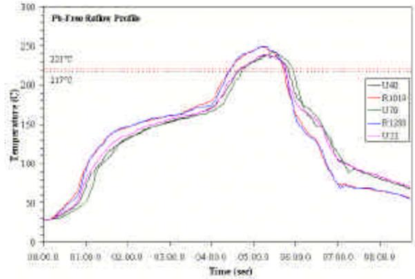
**Figure 3 - Reflow Profile Used for all Pb-Free Pastes**
