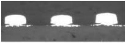
**Figure 6 - Under Cut with Conventional Soft Etching Solution**
