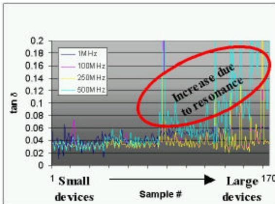
Figure 9 – CFP Loss Tangent at Various Frequencies
