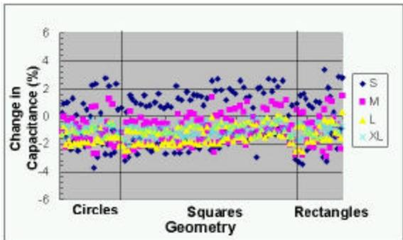
**Figure 12 – Change in CFP Capacitors Following 5X Reflow and 1000 Cycles LLTS**
