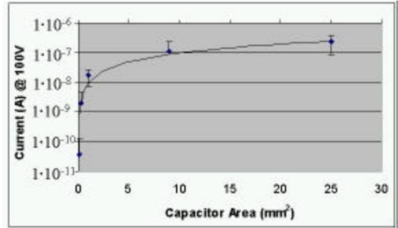
Figure 10 – Capacitor Leakage Current vs. Area
