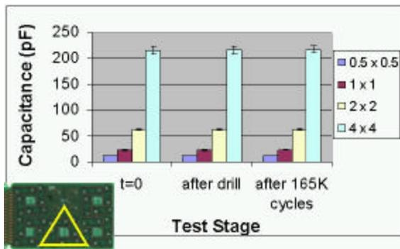
**Figure 15 – Capacitance Change Following Bend Testing; Inset Shows Support Points**
