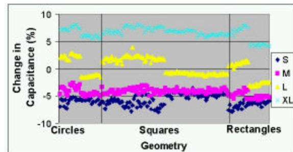
**Figure 14 - Change in CFP Capacitors Following 5X Reflow and 250 Hours 85°C/85%RH Storage**
