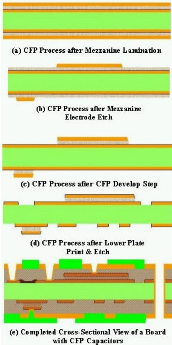
Figure 2 – CFP Dielectric Fabrication Process
