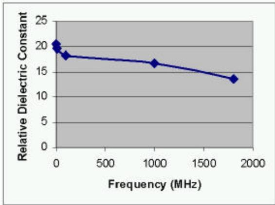
Figure 8 – D<sub>k</sub> vs. Frequency
