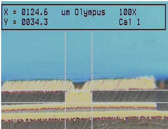
Figure 3 - Microscope Cross Section of CFP Capacitor with Mezzanine  $\mu$ via Contact
