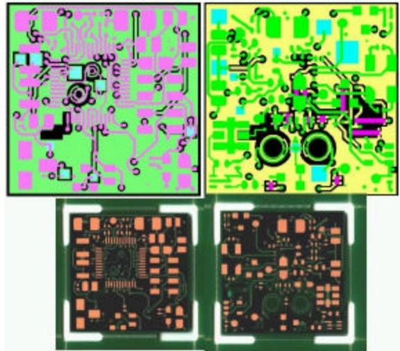
**Figure 16: Layout & Photos of a RF Module Incorporating CFP Capacitors**
