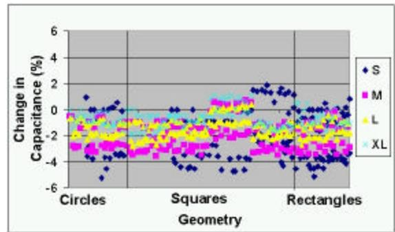
**Figure 13 – Change in CFP Capacitors Following 5X Reflow and 1000 Cycles AATC**
