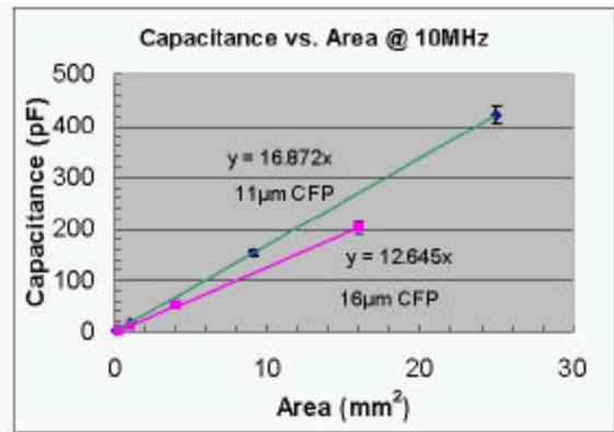
Figure 6 – Capacitance vs. Area
