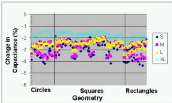
**Figure 11 – Change in CFP Capacitors Following 5X Reflow**
