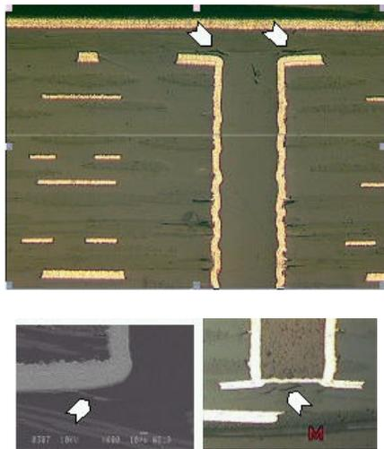
**Figure 17 – Laminate Cracks Between the Via Fill Material and Prepreg Outside the Buried Core Via**
