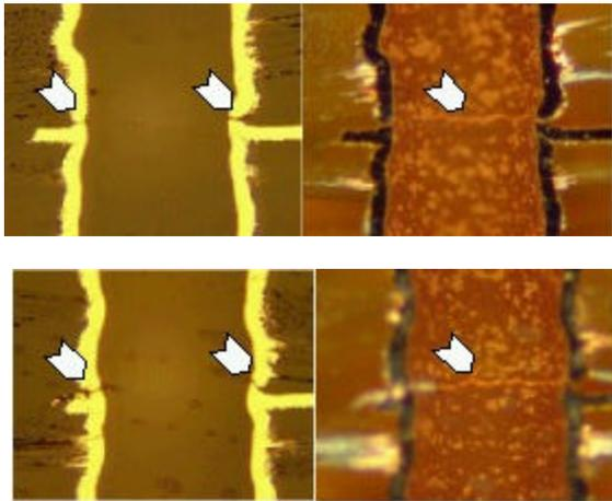
**Figure 16 - Barrel Cracking in Buried Core Vias Filled with Resin from Prepreg during Final Lamination (Left: Bright Field, Right: Dark Field)**
