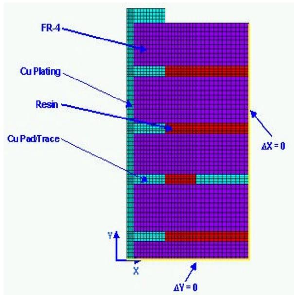
**Figure 3 – Finite Element Model of PTH**
