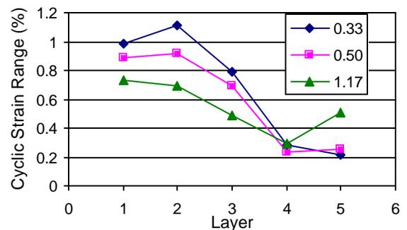
**Figure 6 – Variation of the Cyclic Strain Range at the Pad/Barrel Interface (PTH Diameter in mm)**
