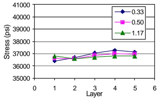
**Figure 10 – Variation of Von Mises Stress at the Pad/Barrel Interface (PTH Diameter in mm)**
