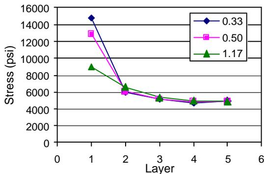
**Figure 9 – Variation of Shear Stress in the XY-Direction at the Pad/Barrel Interface (PTH Diameter in mm)**
