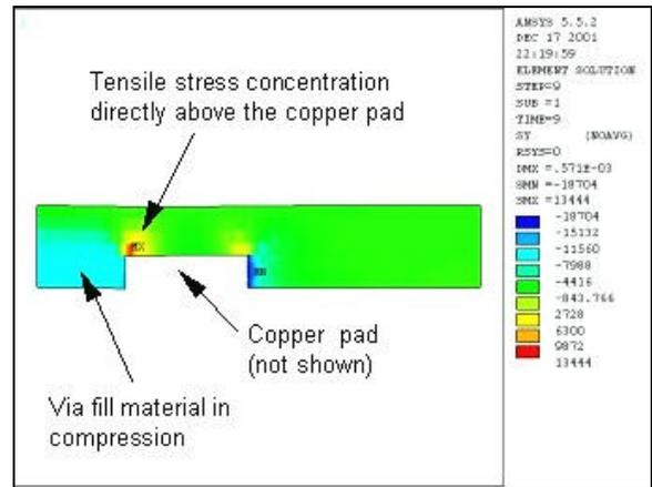
**Figure 18 – Stresses (Y-Direction) Distribution in the Dielectric Layer over the Buried Via During the Heating Cycle**
