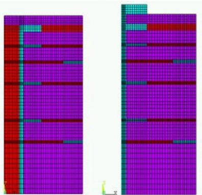
**Figure 12 – FE Model of A 14 layer PWB with Buried Core Via (Left) and PTH (Right)**
