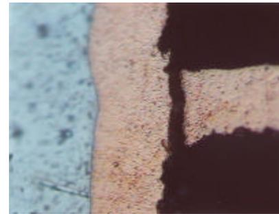
**Figure 5 – Post Separation at a Backplane Connector Hole After Assembly**
