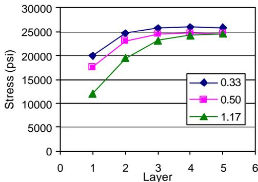
**Figure 8 – Variation of Stress in the Y-direction at the Pad/Barrel Interface (PTH Diameter in mm)**
