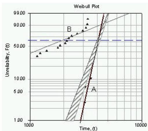
Figure 2 – Weibull Plot Showing the 2<sup>nd</sup> Level Reliability of Different Reliability Packages and PTH
