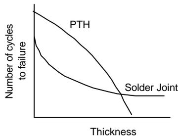
Figure 1 – Effect of Board Thickness on PTH and Solder Joint Reliability
