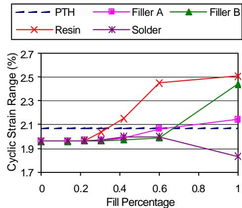
**Figure 13 – Maximum Cyclic Strain Range in a Buried Core Via with Different Via Fill Materials and Fill Percentage**
