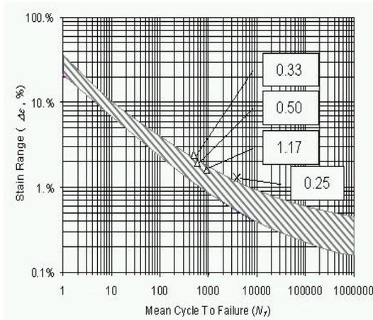
**Figure 4 – Comparison of PTH Fatigue Models (shaded area) with Experimental IST Data of 3 PTH Sizes (D) and ATC data (X)**
