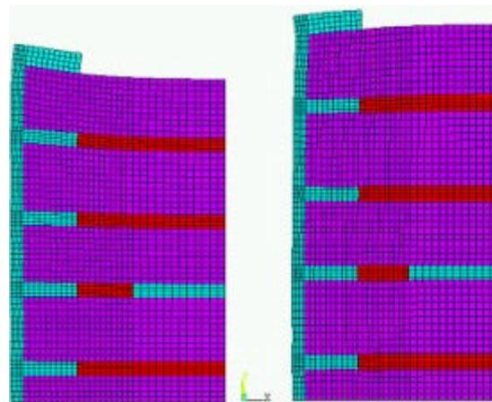
**Figure 11 – Bending of the PTH Pads (Pad Rotation) During Thermal Loading (Left: Cold Cycle; Right: Hot Cycle) Note: Deformation is Exaggerated by About 7X**
