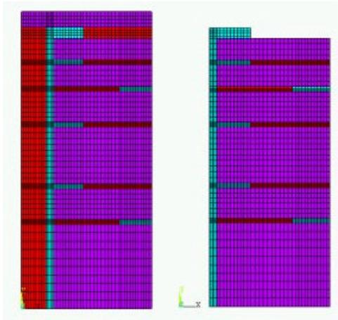
**Figure 14 – A Buried Core Via (left) vs. A PTH (right) of the Same Aspect Ratio**
