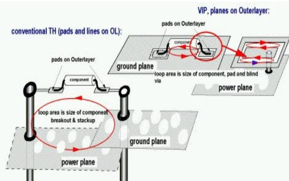
**Figure 4 - Comparison of the Power-ground Loop on a Conventional through-hole Multilayer Compared to a Microvia-in-pad Design with a Flooded Surface Ground Plane**
