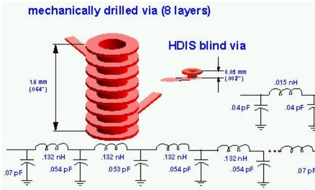
**Figure 3 - Lumped Models of a Microvia Compared to a Drilled Through-hole Via**
