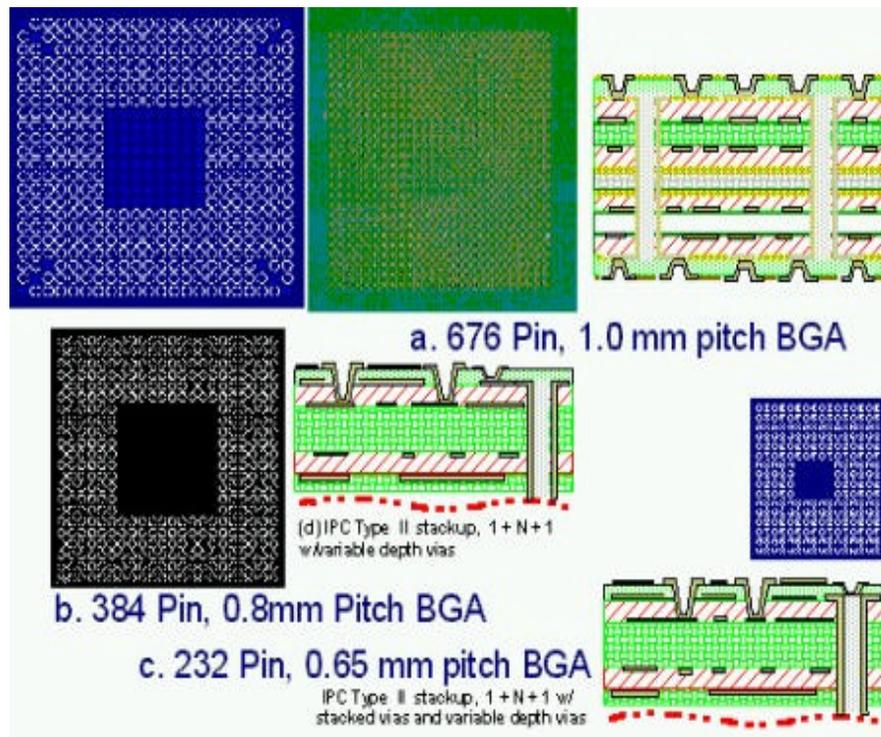
**Figure 6 - Three Fine-pitch BGAs that Require Microvias:**
