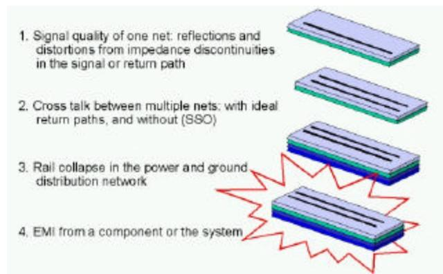
Figure 2 - All Signal Integrity Problems Can Be Grouped in Four Families
