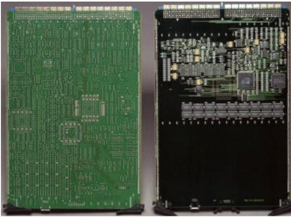
**Figure 5b - The Secondary Side of the Redesigned Multilayer Shows the Advantage of Blind Vias and the Via-in-pads Design Concept**
