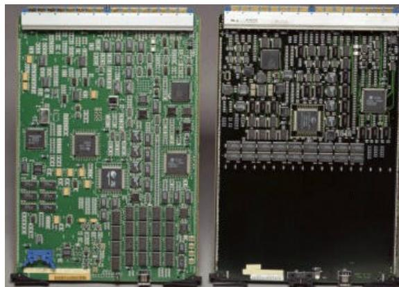
**Figure 5a - A 12 Layer, Controlled Impedance Multilayer was Redesigned Employing only Microvia-in-SMT Pads on the Left is the Original Through-hole Version, and on the Right, the Microvia Version but Requiring only 8 Layers**
