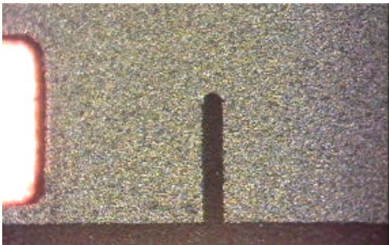
**Figure 1 – Single Plunge Cut Laser Trim for Thin Film 50 Ohm Resistor**
