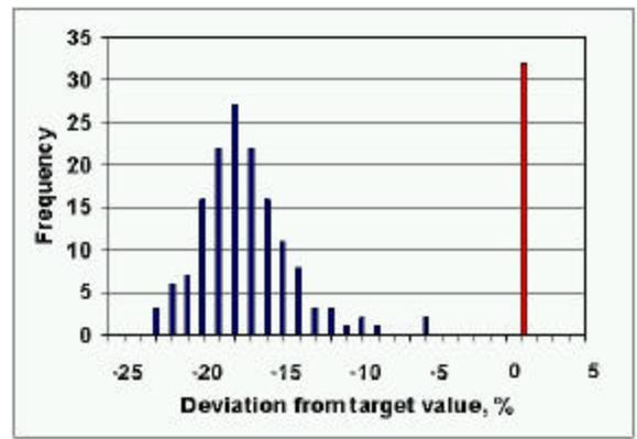
**Figure 14 – Distribution of Printed Resistor Values before Trimming (Black) and after Trimming (Red) Relative to the Target Value**
