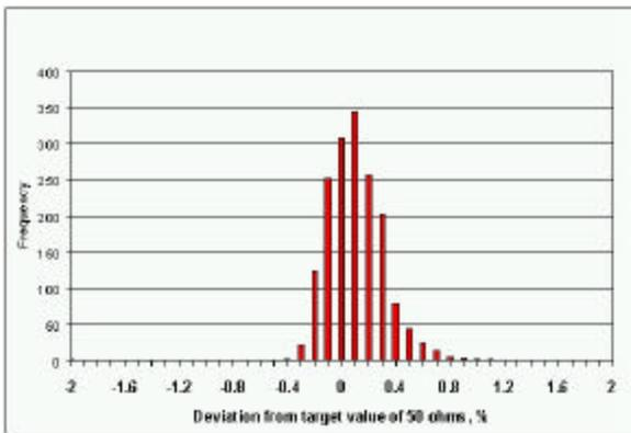
**Figure 5 – Expanded View of the Final Distribution of Resistor Values after Trimming**
