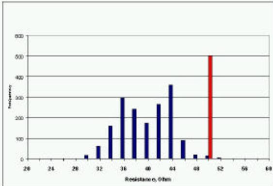
**Figure 4 – Pre-Trim (Blue Bars) and Post-Trim (Red Bar) Values for Laser Trimmed Thin Film Resistors - the Target Value is 50 Ohms.**
