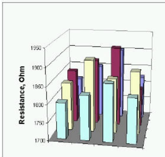
**Figure 13 – Distribution of resistor Mean Values Across 18x24” Panel for Resistors of Paste B before Trimming**
