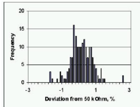
**Figure 11 – Final Values Distribution for a Single Plunge Cut on the Paste with High Sheet Resistivity**
