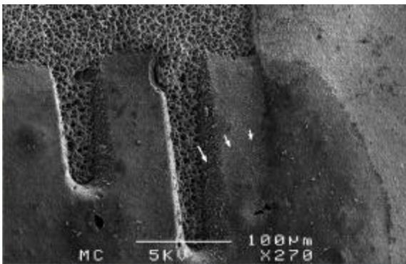
**Figure 9 – Scanning Electron Microscope (SEM) Image of Laser-Trimmed PTF Resistor**
