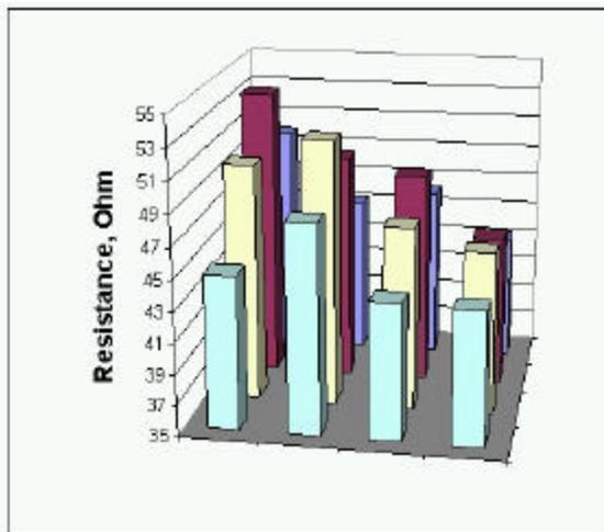
**Figure 12 – Distribution of Resistor Means Values Across 18x24” Panel for Resistors of Paste ‘A’ before Trimming**
