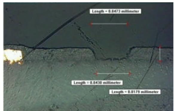
**Figure 8 – Cross-Sectional View of the Laser Trim Cut in a PTF Resistor**
