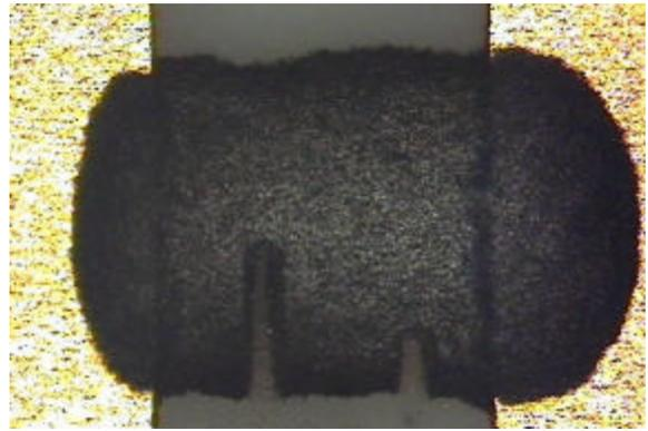
**Figure 6 – Thick Film Resistor with Double Plunge Cut**
