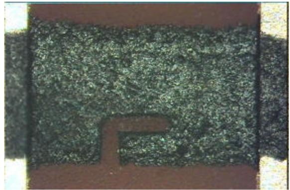
**Figure 7 - PTF Resistor Trimmed with L-Cut**
