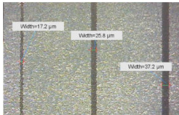
**Figure 2 – Trim Cut Widths of 17μm, 26μm and 37μm on a Thin Film Resistor by Varying Laser Power**
