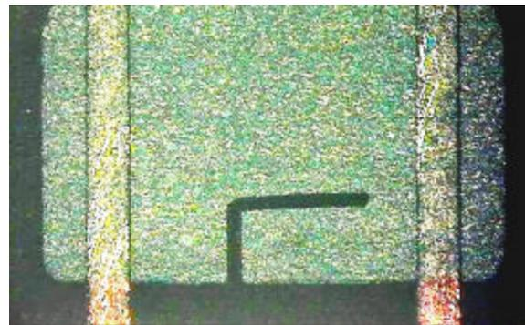
**Figure 3 – Thin Film Resistor Laser Trimmed with an L-Cut**
