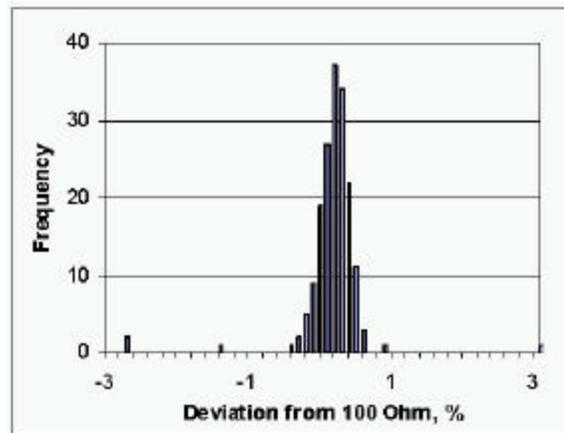
**Figure 10 – Trimming Results for Single Plunge Cut on Low Sheet Resistivity Paste**
