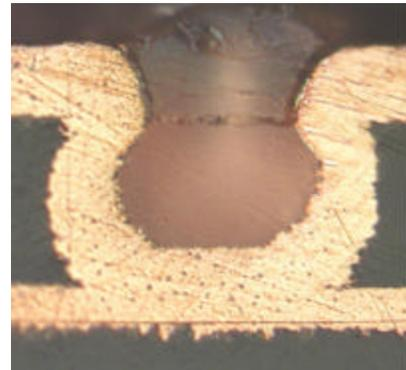
Plating result with production system showing good micro -via throwing power but some slight rough deposit at the base.
