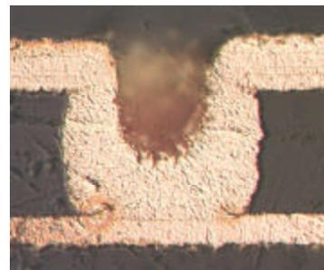
Plating parameters 4 A/dm<sup>2</sup> forward, 30 A/dm<sup>2</sup> reverse. Via filling effect achieved by use of lower effective current density.
