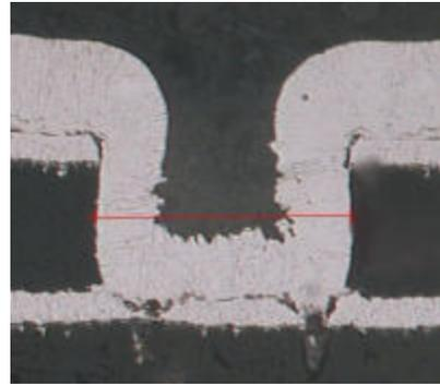
The plating result shows copper plating with the beginning of rough plating even at the relatively low current density used.
