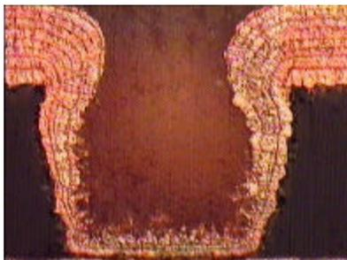
Very poor copper deposit showing typical mass transport limitations "burnt" copper plating.
