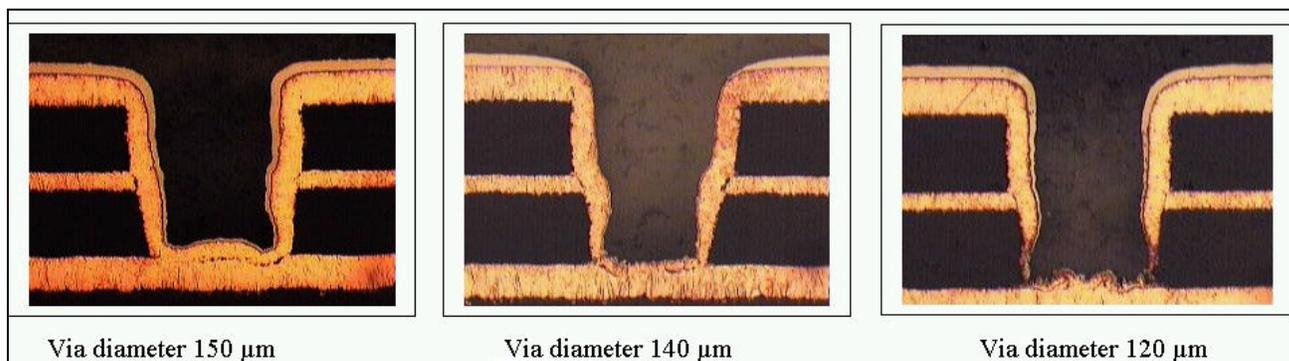
Figure 1 - Effect of the Increase in Blind Micro-Via Aspect Ratio on Copper Plating Quality
