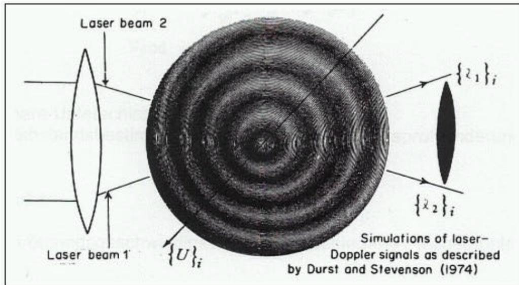
Figure 3 - Schematic Operation of an LDA Measurement System
