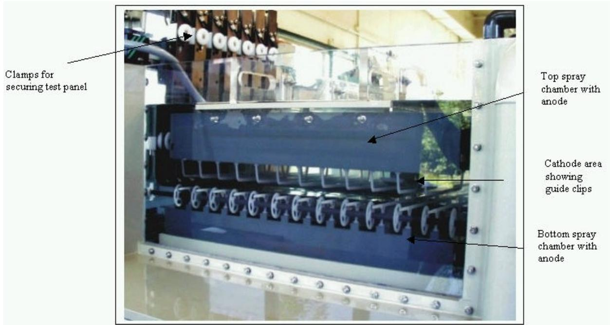
Figure 2 - Side View of Idealized Horizontal Plating Cell
