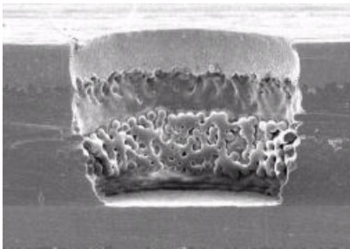
**Figure 4 - Laser Drillable 1080 Fabric 500X**
