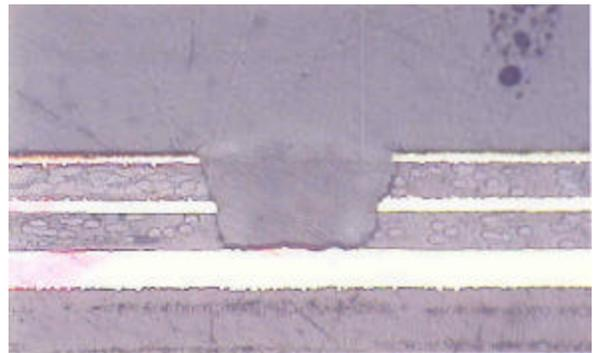
Figure 1 – Microvia Using YAG/CO<sub>2</sub>
